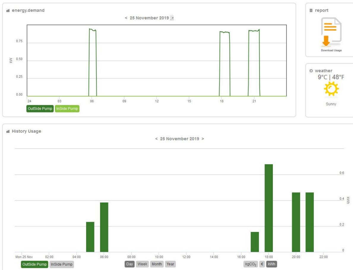
Figure 42. Extreme daily function of Pump C2 on 25/11/2019 (heavy rain event).
