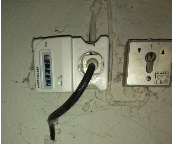
Figure 5. Power consumption measurements of existing water pumps in Building B (Pump B1 on the left and Pump B3 on the right, photo taken on 22/07/2019).
