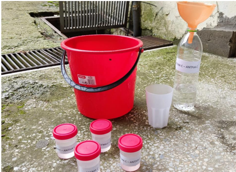
Figure 54. Sampling procedure for chemical and microbiological analysis (pump C2)
