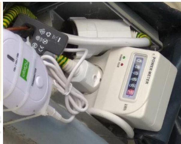
Figure 6. Power consumption measurements of existing water pumps in Building C (Pump C1 on the left and Pump C2 on the right, photo taken on 22/07/2019).
