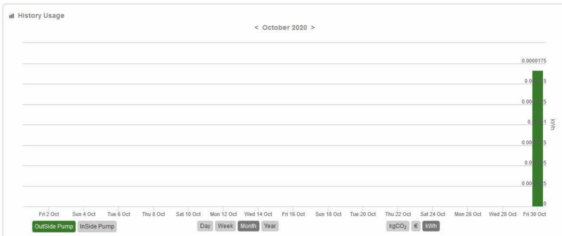
Figure 26. Diagram of history power usage (in kWh) of Pump C2 (October 2020).
