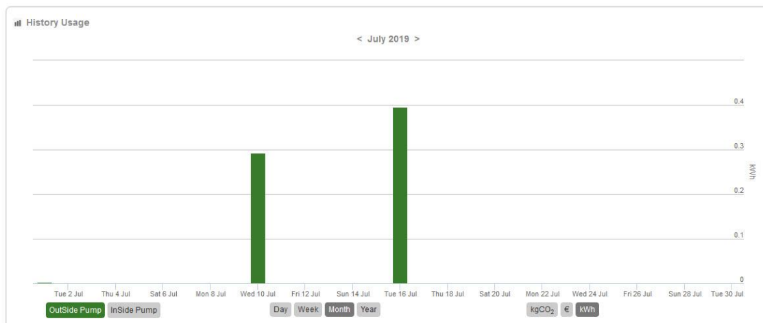
Figure 11. Diagram of history power usage (in kWh) of Pump C2 (July 2019).
