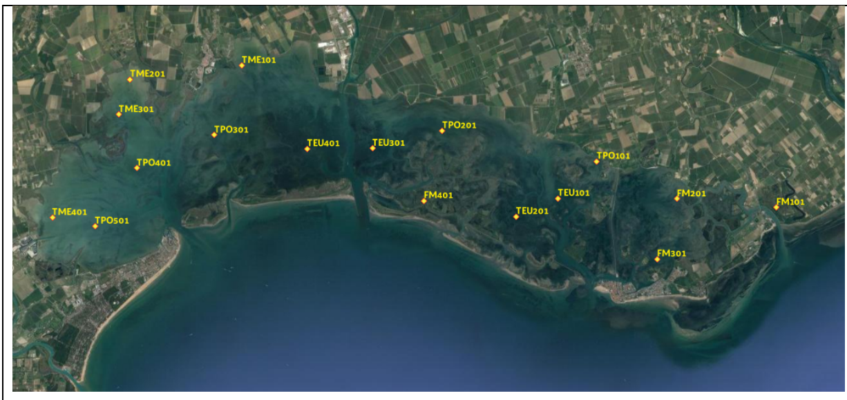
Fig. 2.2.2 Monitoring network for the quality of transitional waters in Grado and Marano Lagoon
