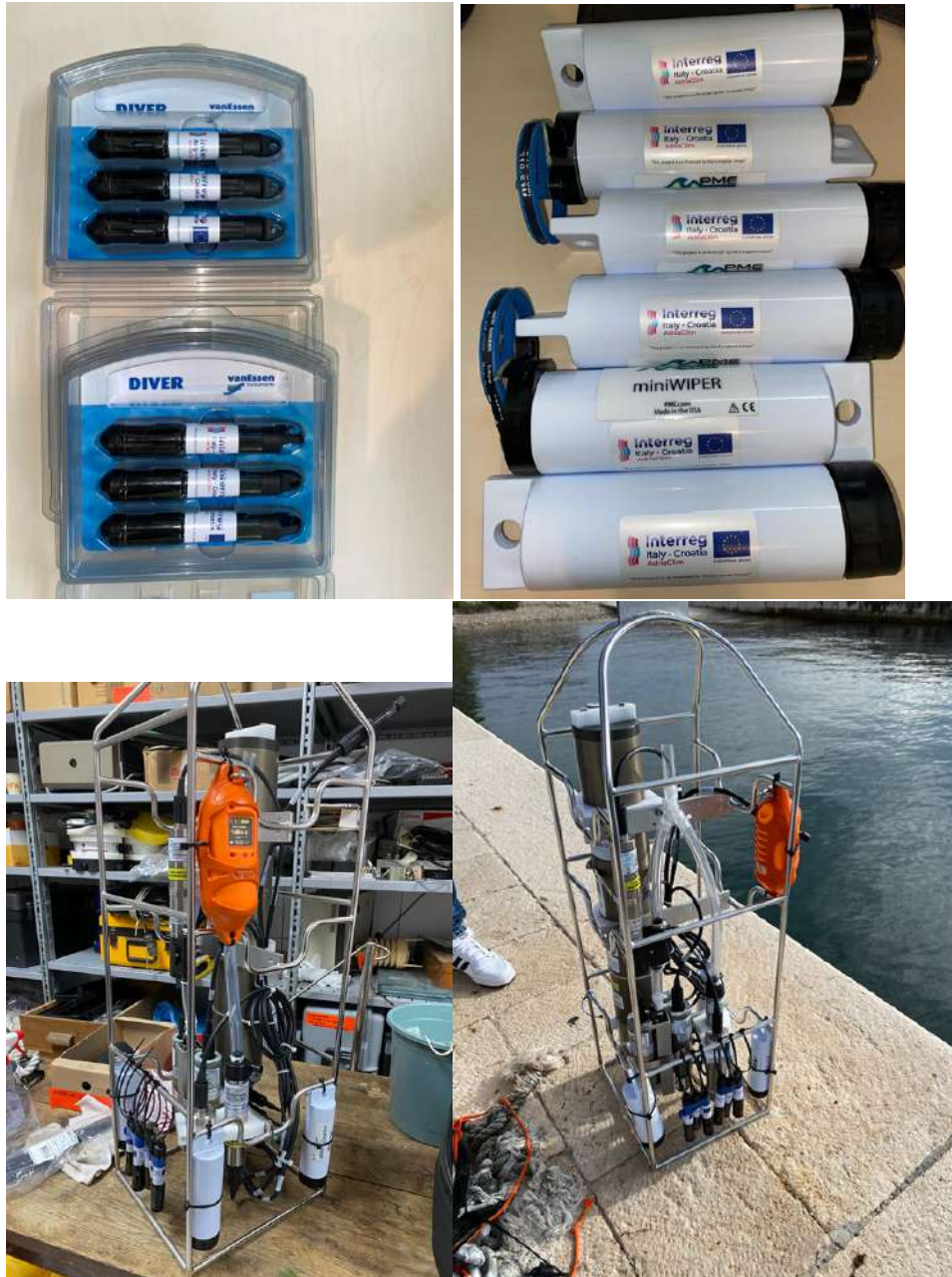
Figure 25. Autonomous sensors for continuous measurements in the Neretva River estuary: CTD sensors (upper left) and dissolved oxygen sensors with wipers (upper right). Testing of sensors using CTD probe: installation of sensors on the probe in the laboratory (lower left) and measurements in front of the IOF building (lower right).
