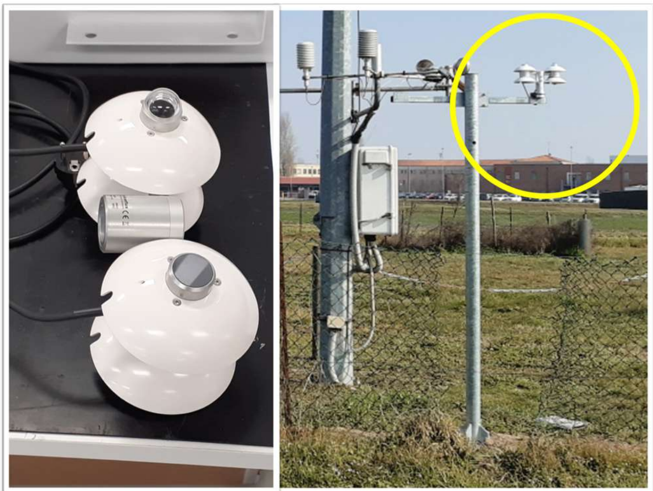
Figure 10. 4-component radiometer before installation (left) and installed in Legnaro PD (right).
