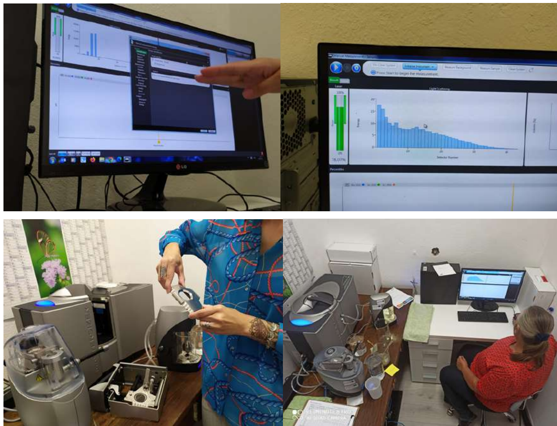
Figure 29. Laboratory work with laser grain size analyser (MASTERSIZER).
