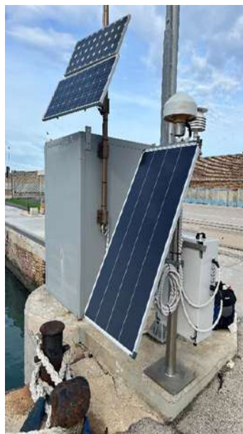
Ortona GNSS station [ID: OTNA domes number: 14678M001]
