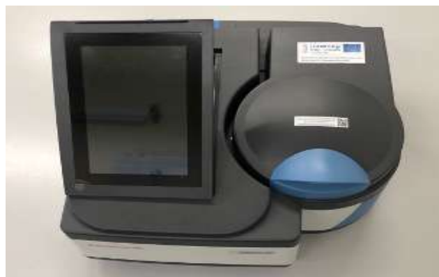
Figure 20. UV-VIS Genesys™ 180 Spectrophotometer (Thermo Fisher Scientific) (UNIBO-CIRSA).
