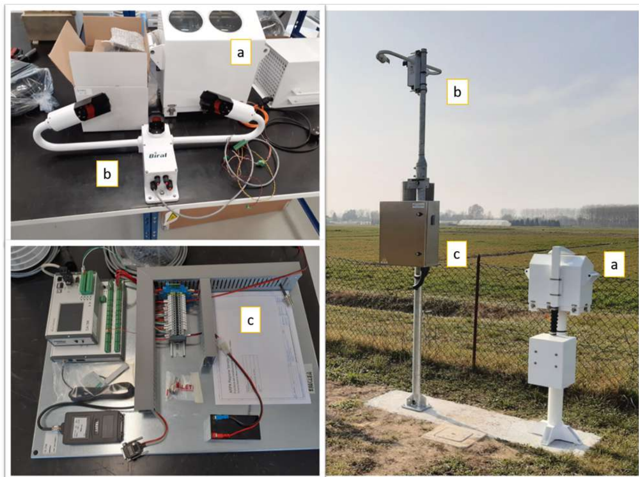
Figure 9. Nephoipsometer (a), present time sensor (b) and data acquisition and transmission system (c) before installation (left) and installed in Legnaro station PD (right).
