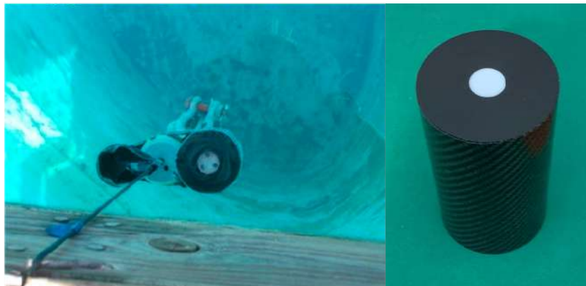
Figure 23. Prototype of a new low-cost multispectral radiometer
