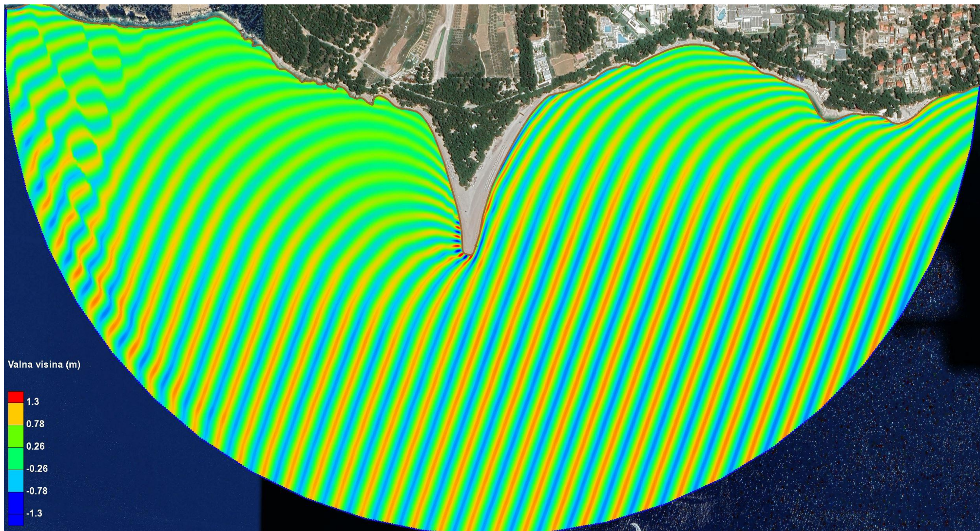
Figure 6.22 – Current wave outline for simulation A1 – the existing state of Zlatni rat beach (Brač) with wave parameters from the direction of ESE (112.5°), 50-year return period ( H_s=2.41 )
