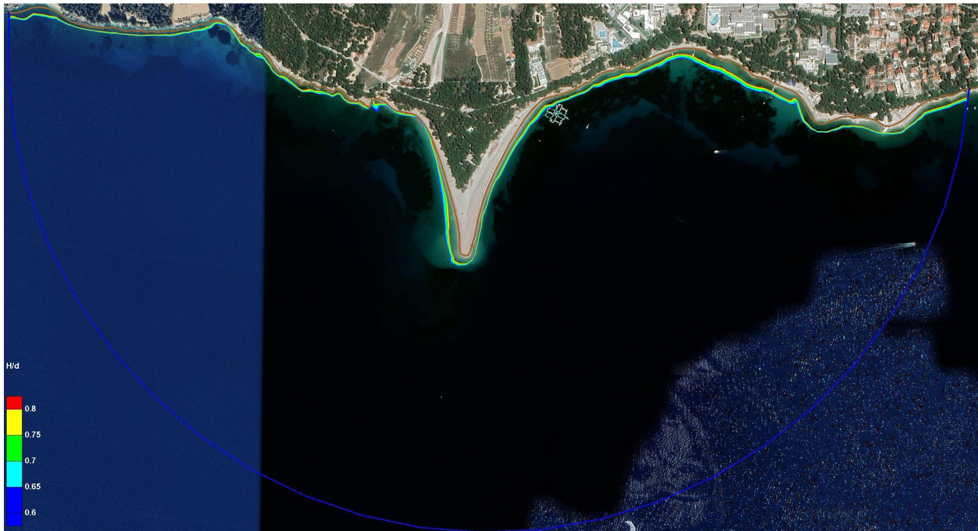
Figure 6.29 – Wave breaking zone for simulation A6 – the existing state of Zlatni rat beach (Brač) with wave parameters from the direction of SSE (157.5°), 50-year return period ( H_s=2.05 m; T_p=5.84 s) and sea level corresponding to absolute maximum
