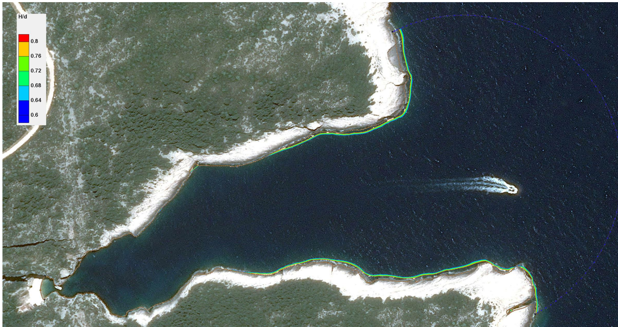
Figure 6.40 – Wave breaking zone for simulation A9 – existing state of Stiniva beach (Vis) with wave parameters from the direction of SE ( 135^\circ ), 50-year return period ( H_s=4.81 m; T_p=8.94 s) and sea level corresponding to middle sea level (SRM)
