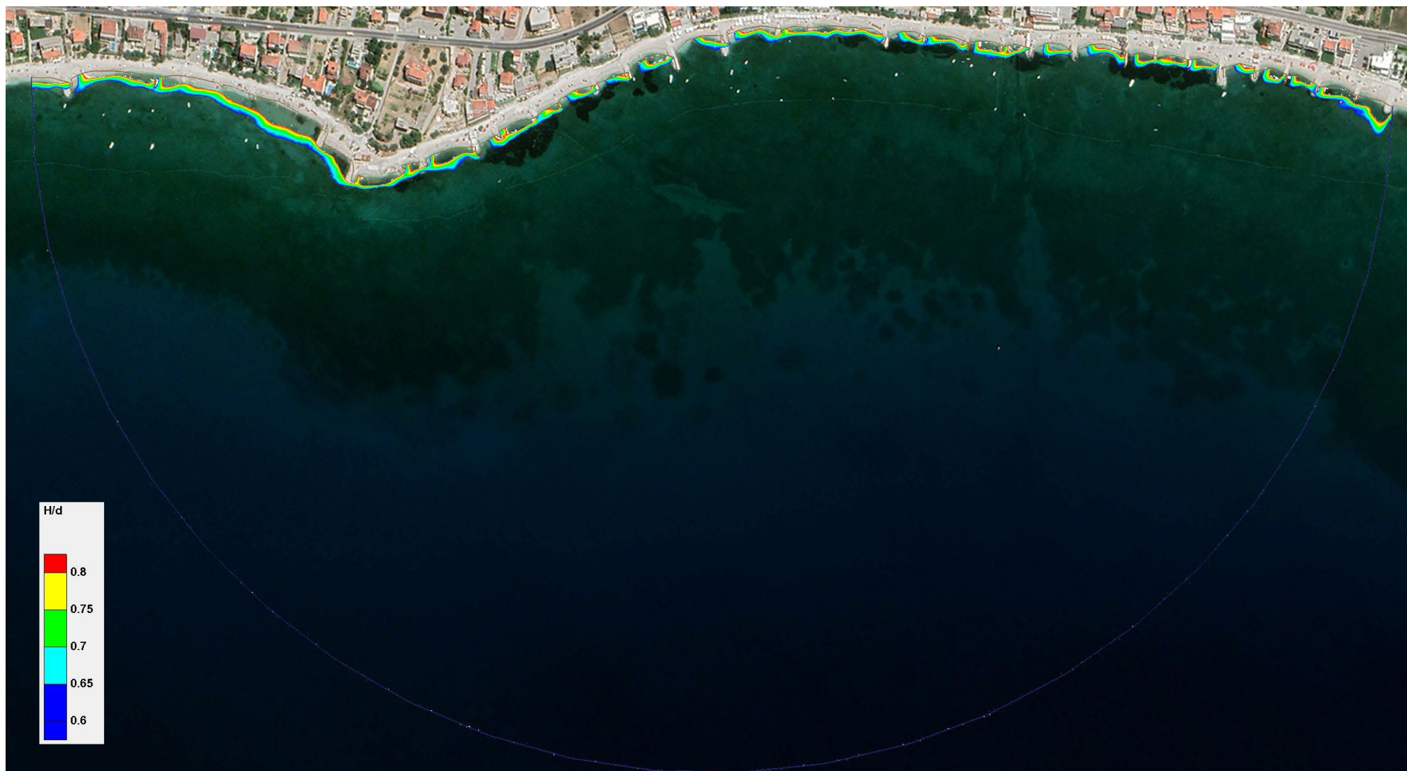
Figure 6.67 – Wave breaking zone for Simulation A23 – the existing state of the beach on the Podstrana-Duče area with wave parameters from the direction W (270°), a 50-year return period ( H_s=1.73 m; T_p=5.36 s) and a sea level corresponding to the absolute maximum
