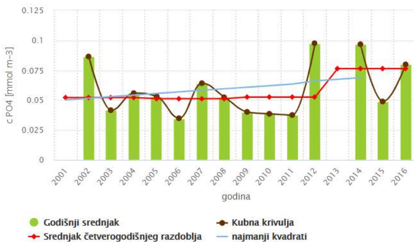
Figure 128. Average annual values of orthophosphate concentration in the surface layer of Cetina estuary (in order of appearance: annual mean, the mean of a four-year period, cubic curve, smallest squares).
