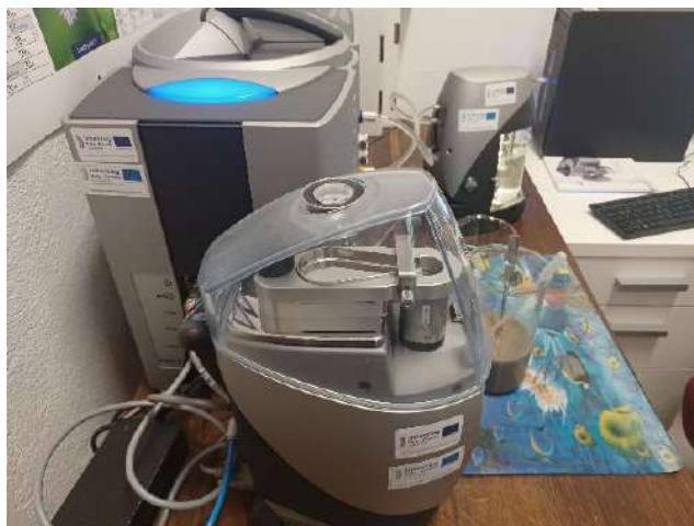
Figure 25. Laser granulometer (Malvern Panalytical Mastersizer 3000 E + Hydro EV + Hydro M).
