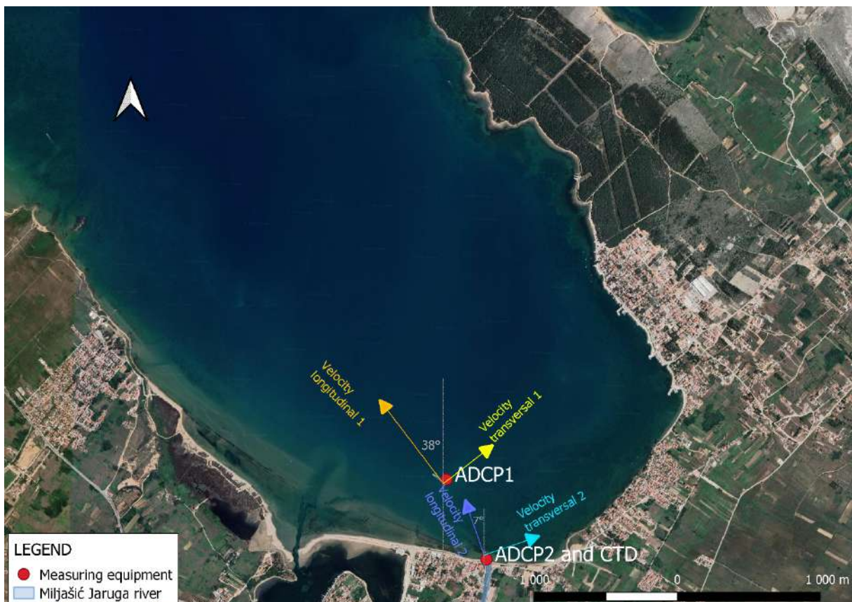
Figure 32. Schematic of the longitudinal and transversal velocity components for ADCP1 and ADCP2 location presented in plain view of the study area.
