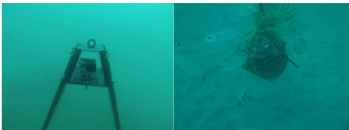
Figure 27. BRUV method (Baited remote underwater video)
