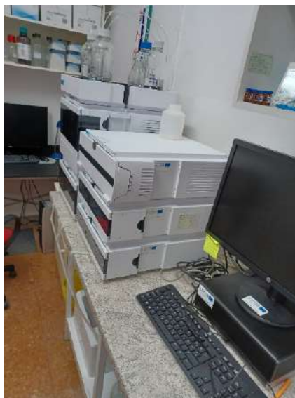
Figure 22. Ultra-high performance liquid chromatograph (UHPLC, Agilent 1290 Infinity II Fluorescence Detector)
