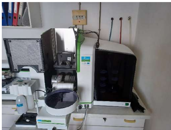
Figure 24. Atomic absorption spectrometer (AAS, PinAAcle 900T, PerkinElmer)
