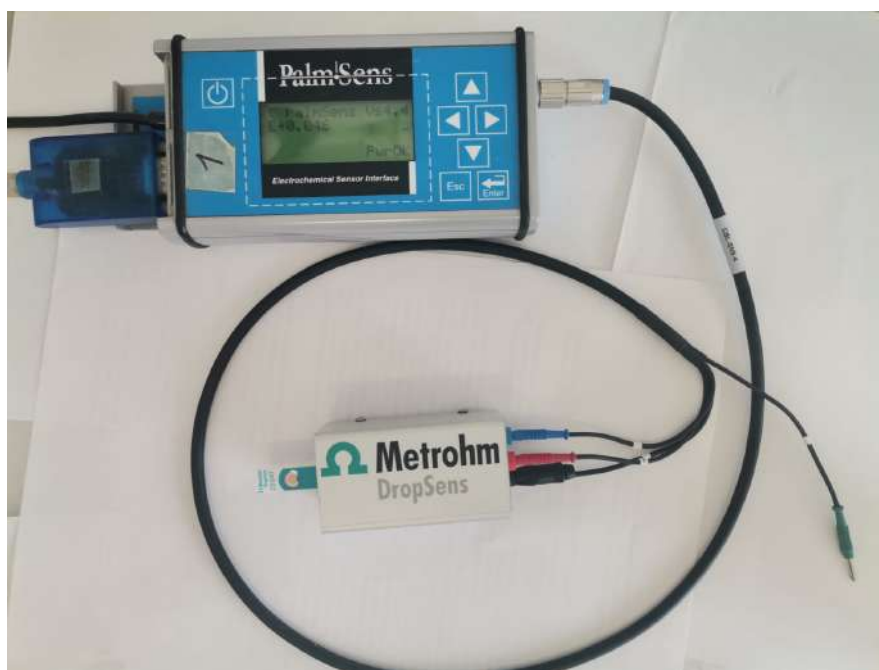
Figure 21. Potentiostat PalmSense 4 equipped with a cable connector for (disposable) screen-printed electrodes
