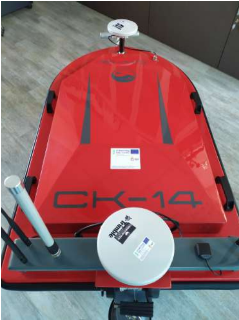
Figure 16. Unmanned Surface Vehicle for hydrographic and environmental survey
