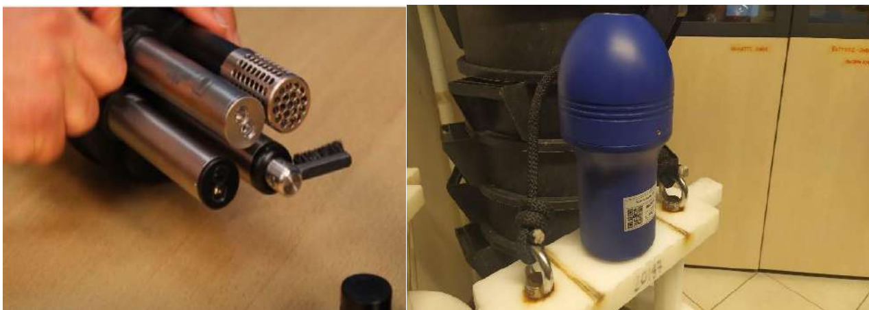
Figure 2. The probes equipped with 3 sensors and the wiper in the center on the left and the GPS/GPRS modem connected on the right
