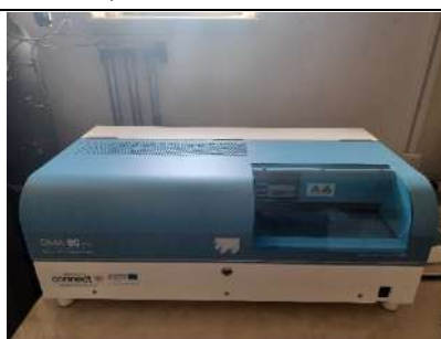
Figure 23. Direct mercury analyser (DMA 80, Milestone)
