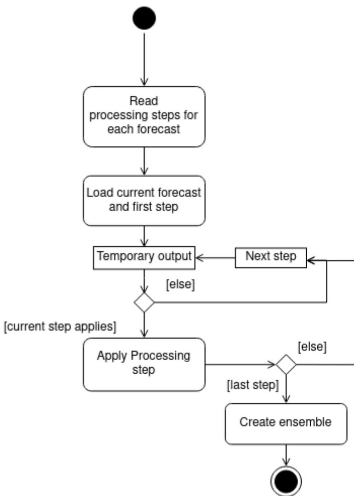
Each forecast has to be processed in a different way: all the possible steps are implemented in the code (e.g. merge or split variables, rename variables, spatial interpolation on the final grid, temporal interpolation, add tide and offset for sea level, invert wave direction and so on). The processing steps and relative parameters required for each forecast are declared in the configuration files as a JSON object.
