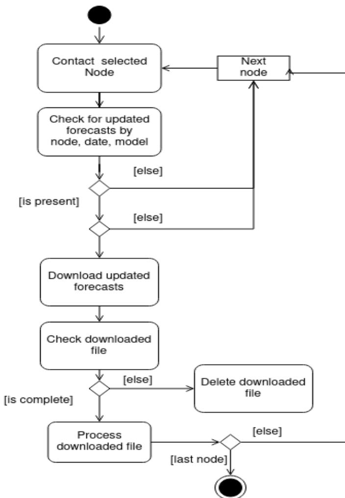
The diagram of the download stage of MMES software is shown in Figure 1. The Daily forecasts are usually published in the morning, but they are not available at the same time and therefore the software contacts all source nodes at regular intervals and checks if the current file is available. If the file is already downloaded and processed the software will pass to the next node.
