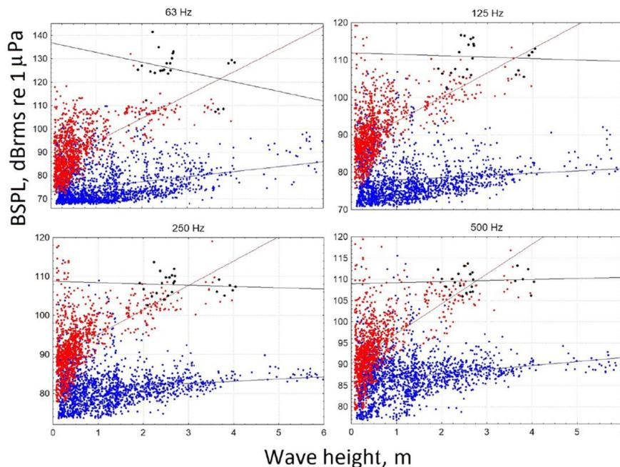
Figure 27. Some examples of scatter plots for band sound pressure level (BSPL) versus wave height at different frequencies recorded at the Pantelleria test site. Blue = before installation; red = after installation; black = during operation (source: Buscaino et al. 2019).
