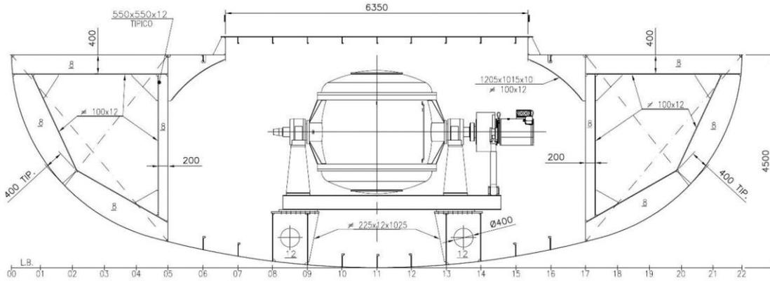
Figure 9. Cross section of the 100-kW prototype (source: Mattiazzo et al. 2014).
