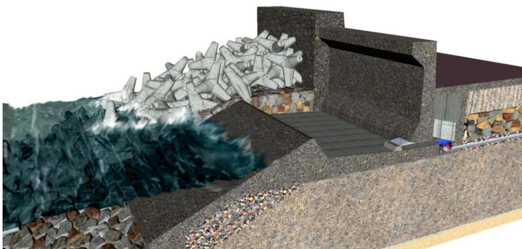
Figure 14. 3D model of a breakwater equipped with OBREC compared to a traditional rubble mound breakwater (source: Palma et al. 2014). The particular configuration at the top of the parapet in the OBREC-equipped breakwater is designed to minimise the water overflow at the back of the structure, compensating for the absence of the traditional rubble mound.
