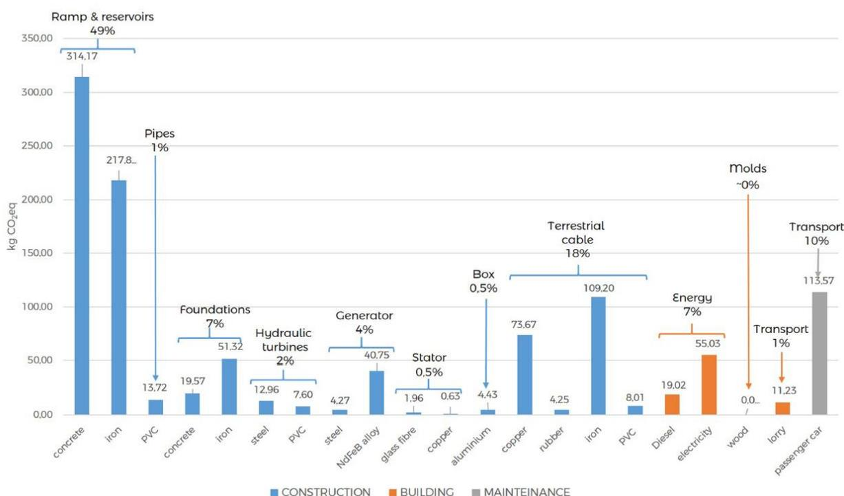
Figure 29. Breakdown of the carbon footprint of the OBREC prototype installed at the port of Naples (source: Patrizi et al. 2019).
