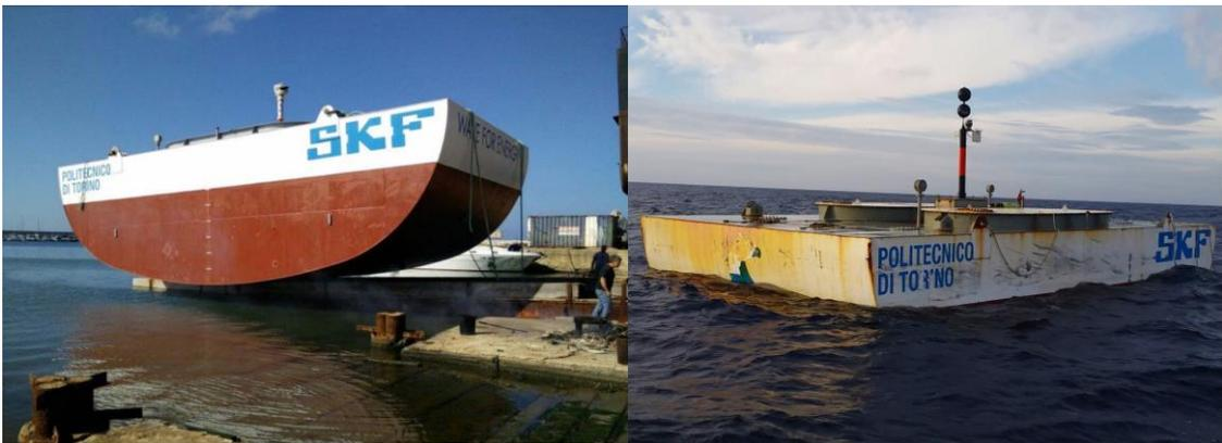
Figure 7. The ISWEC prototype before being towed to Pantelleria (left), and at sea off the island (right) (source: Wave for Energy).
