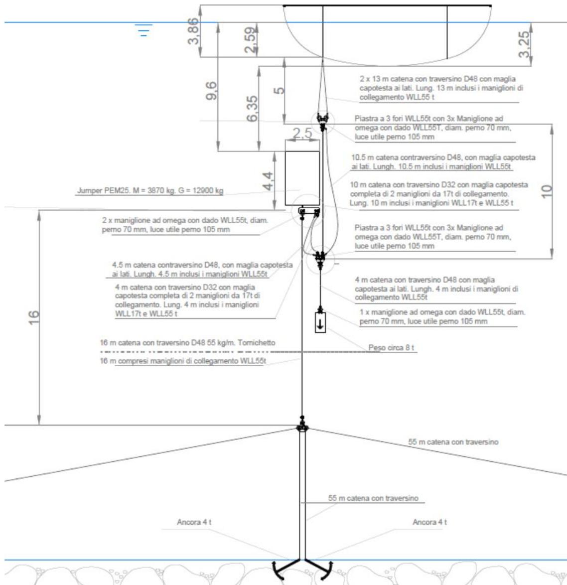
Figure 24. Scheme of the main mooring system for the ISWEC prototype deployed off Pantelleria (source: Mattiazzo et al. 2014).
