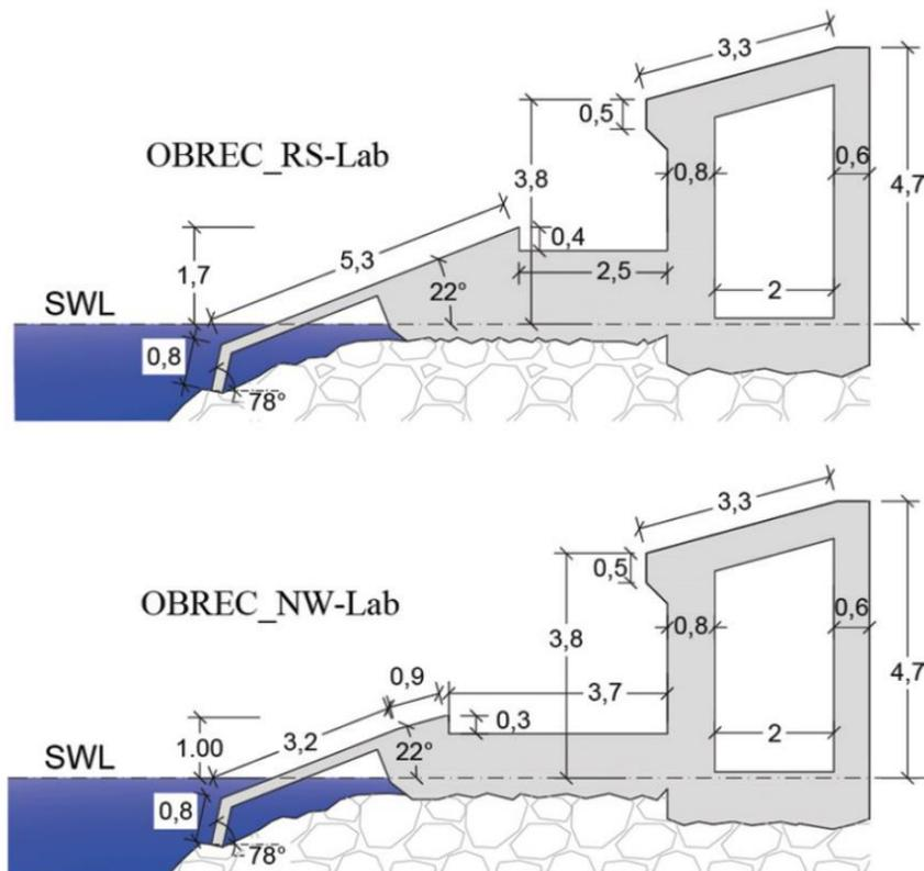
Figure 12. Cross-sections of the OBREC module prototype installed in Naples (source: Di Lauro et al. 2019). In order to test different operating conditions, the module has two parallel reservoirs at different heights.
