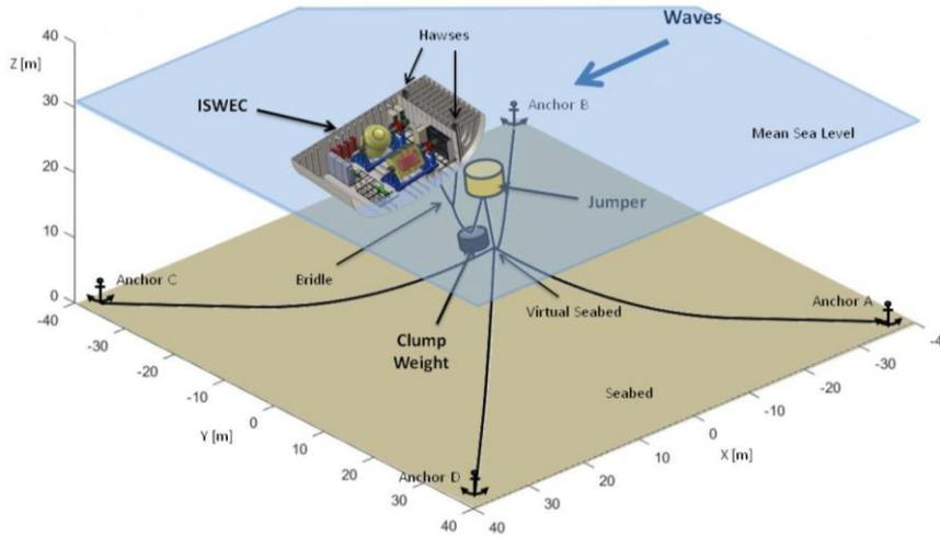
Figure 25. Scheme of the mooring system for the ISWEC prototype deployed off Pantelleria (source: Vissio 2017).
