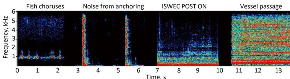
Figure 28. Spectrogram of sounds from fish choruses, noise from the anchoring system after installation, noise from the operating ISWEC, and noise from a vessel passage recorded at the Pantelleria test site (source: Buscaino et al. 2019).
