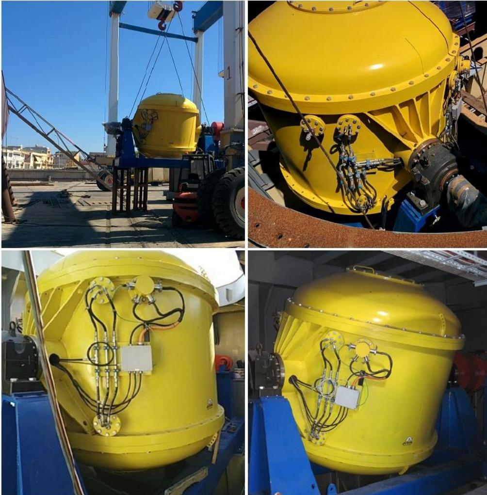
Figure 11. Pictures of one of the gyroscope groups installed on the 100-kW prototype (source: Vissio 2017).
