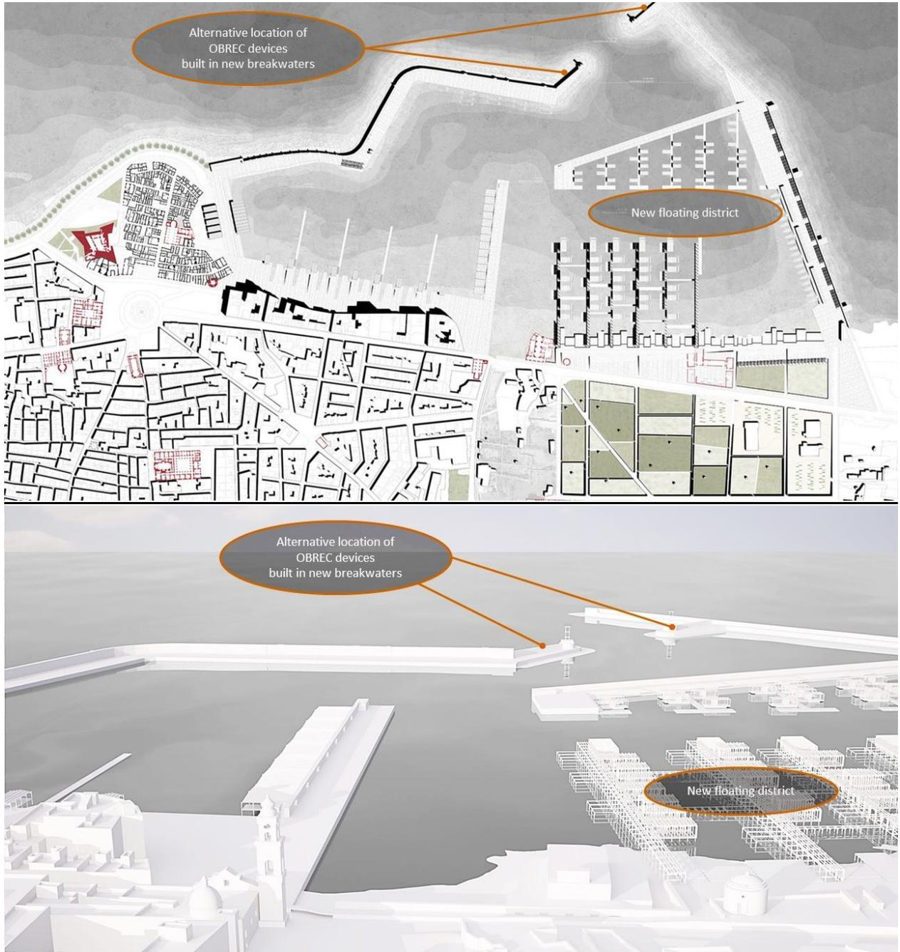
Figure 22. Alternative location for the OBREC devices (source: Michele Montemurro). Their integration in new breakwaters planned for protecting a port expansion would allow to save on costs.
