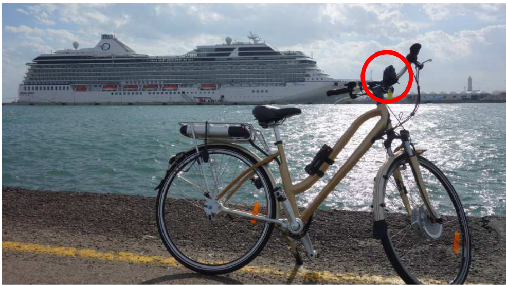
FIGURE 36. PHOTO OF THE GPS SYSTEM INSTALLED ON THE ELECTRIC BIKE IN RAVENNA CRUISE TERMINAL
