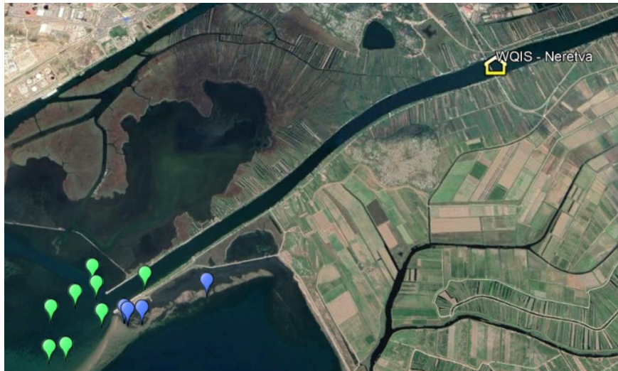
Figure 15. Position of sampling stations: WQIS box (yellow house), sea (blue pin) and river (green pin).
