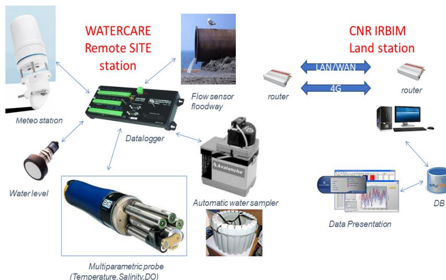
Figure 2. The Block Diagram shows the datalogger connections with sensors, communication stage, centralized database, and web data presentation.
