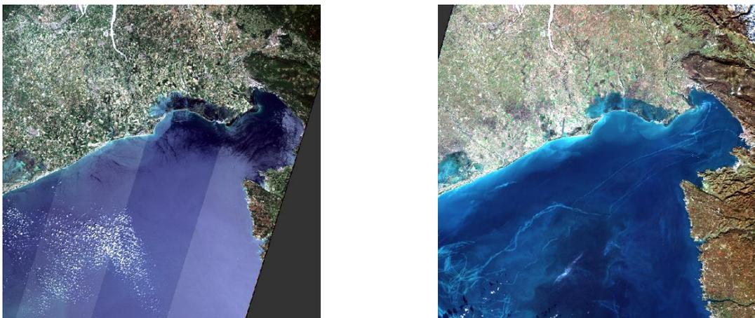
**Figure 4.3.** Comparison between two Sentinel-2 Level 1C tiles displaying the same maritime area with and without sun glint effect disturbance.
