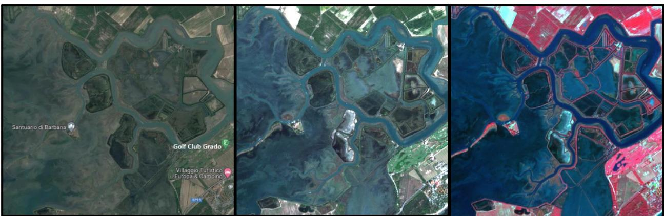
**Figure 4.7.** Eastern part of the Grado Lagoon (Italy) from a Google Maps screenshot. *Left Panel:* RGB image. Each pixel is a combination of the blue band (B02), green band (B03) and red band (B04). Image resolution is 10 m per pixel. *Right Panel:* False colour image. Respect to the RGB image the red band has been replaced with the B08 NIR band. This representation enhance the pixels with high coverage of grass or other plants.
