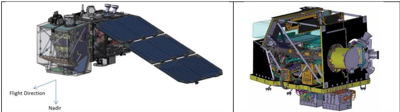
**Figure 2.1.** *Left panel:* schematic view of a Sentinel 2 satellite. The MSI payload is attached on the left of the spacecraft body. *Right panel:* inside view of the MSI instrument. Further details are available through the mission website.
