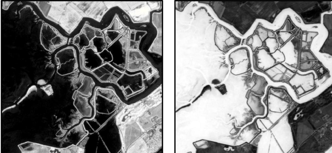
**Figure 4.8.** Indexes maps of Eastern part of the Grado Lagoon. *Left:* NDVI map. Darker areas identify urban or water areas, whiter areas identifies green lands. *Right:* NDWI map. The colour meaning is complementary to the NDVI map, i.e., water bodies are whiter than land.
