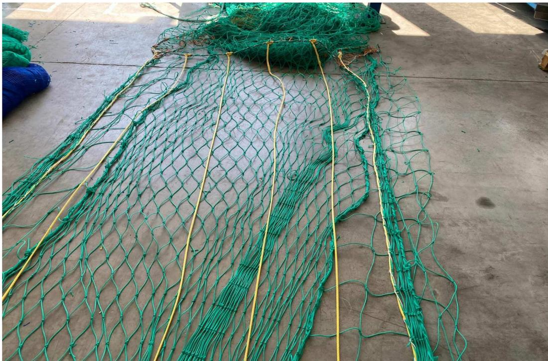
**Figure 2** - Detail of the longitudinal ropes in the upper part of the net.
