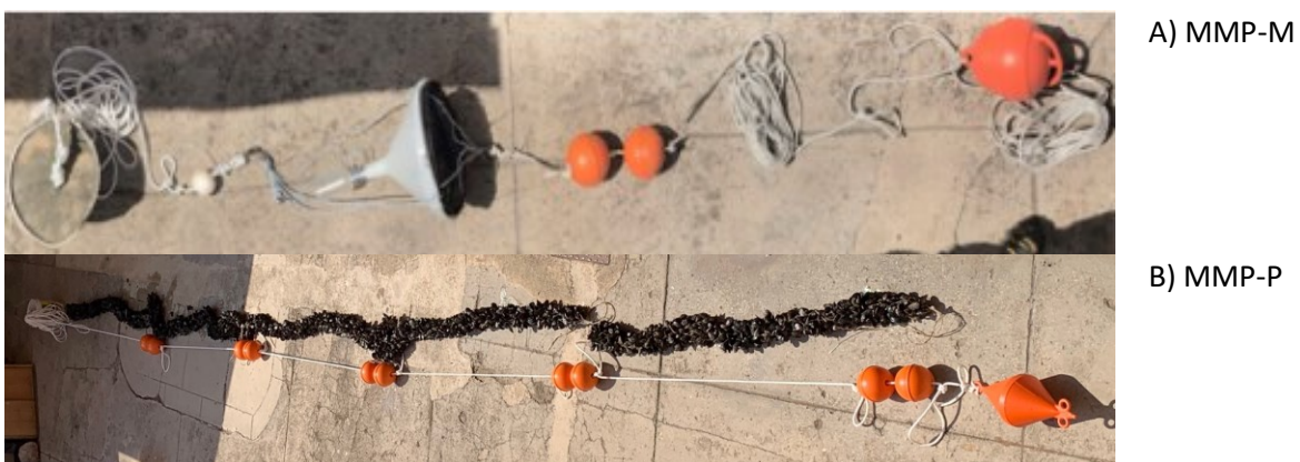
Figure 8: Installations used for A) MMP-M microplastic monitoring in water column and B) MMP-P environment purification.
