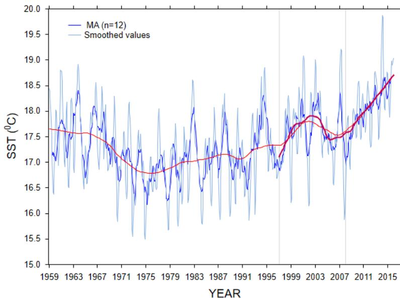
Figure 1. Seasonal decompositions of mean monthly sea surface temperature for the middle Adriatic Sea obtained from moving averages procedure. Non-linear trend for the period 1959–2015 (thin red line) and for the period 1997–2015 (bold red line) are presented as LOWESS spline (obtained from Šolić, Grbec, et al., 2018).
