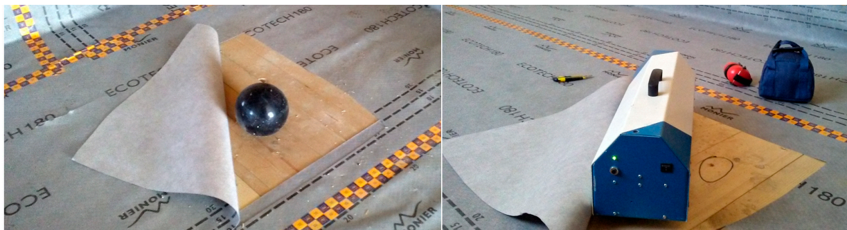
Figure 7. Tapping machine and rubber ball used to test the impact noise of CLT floors.
