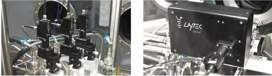
Figure 6.19: An implementation of a substrate/thin film temperature pyrometer (left) and a substrate bow measurement device (right).
