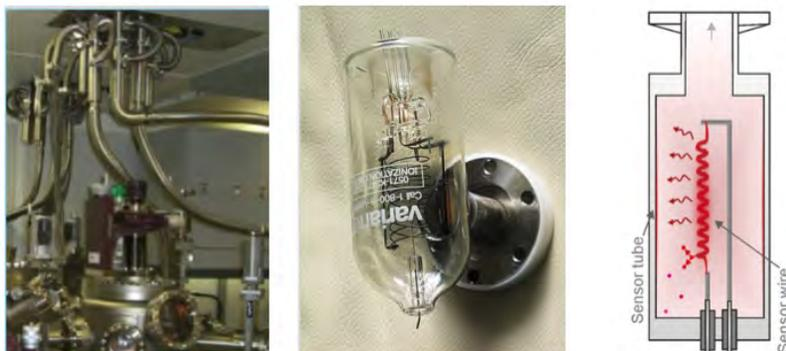
Figure 6.15: Pictures of a liquid nitrogen feed lines coming from a phase separator (left), an ion gauge (middle) and a Pirani gauge filaments (right).
