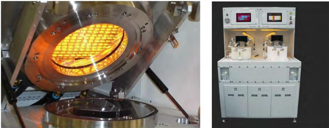
Figure 6.21: A rapid thermal annealing chamber with heating lamps (left) and a wet processing unit to clean wafers (right).
