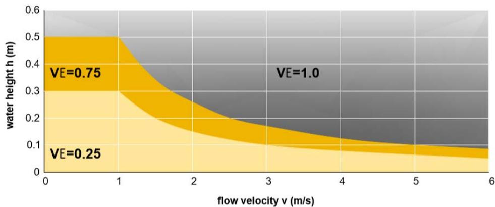
Figure 9: Vulnerability values of network infrastructure as a function of  $h$  and  $v$
