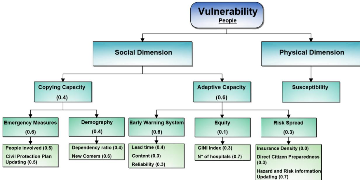
Figure 4: Hierarchical combination of indicators and relative weights
