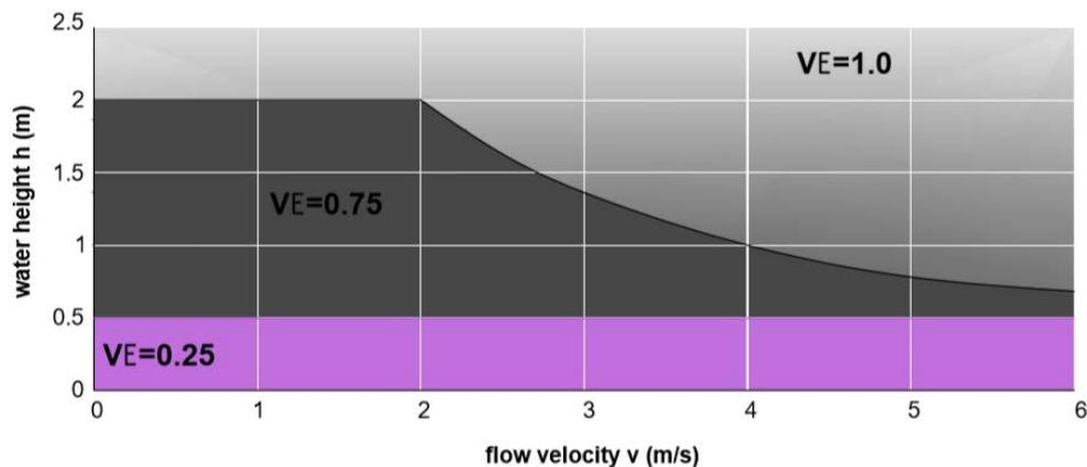
Figure 8: Vulnerability values of buildings as a function of  $h$  and  $v$
