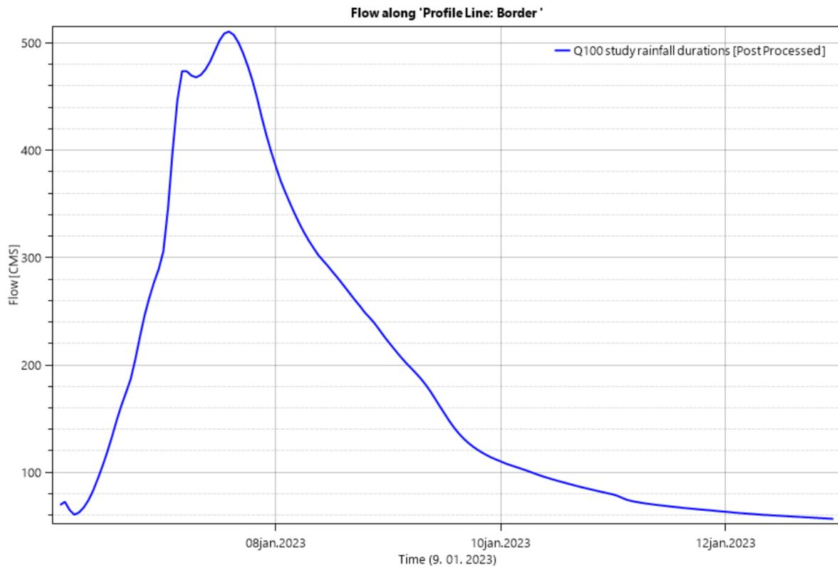
Figure 23: Results of Q100 scenario with updated roughness values at border profile
