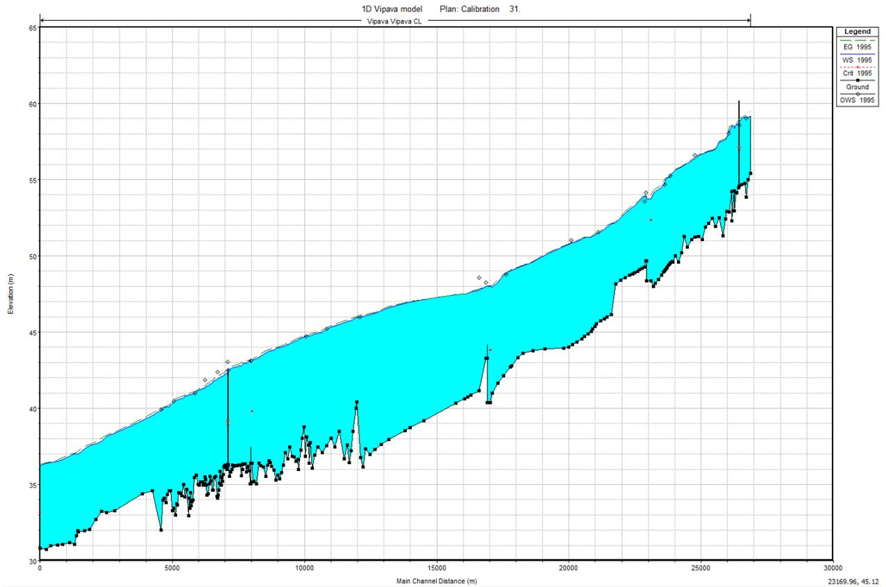
Figure 19: Profile plot of 1D model with calibrated roughness coefficients
