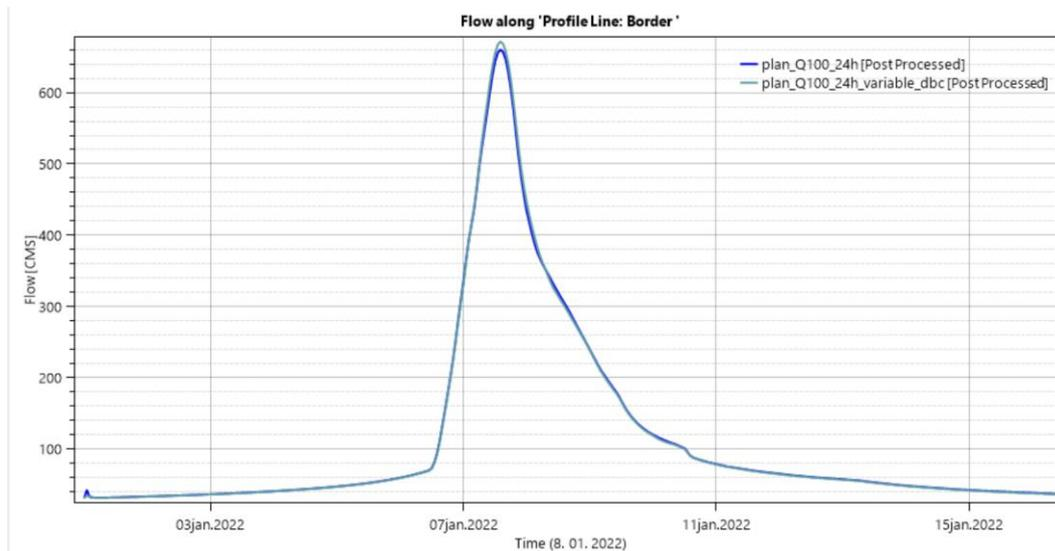
Figure 16: Hydrograph at the border profile showing results of the simulation with 24h rainfall duration input hydrographs
