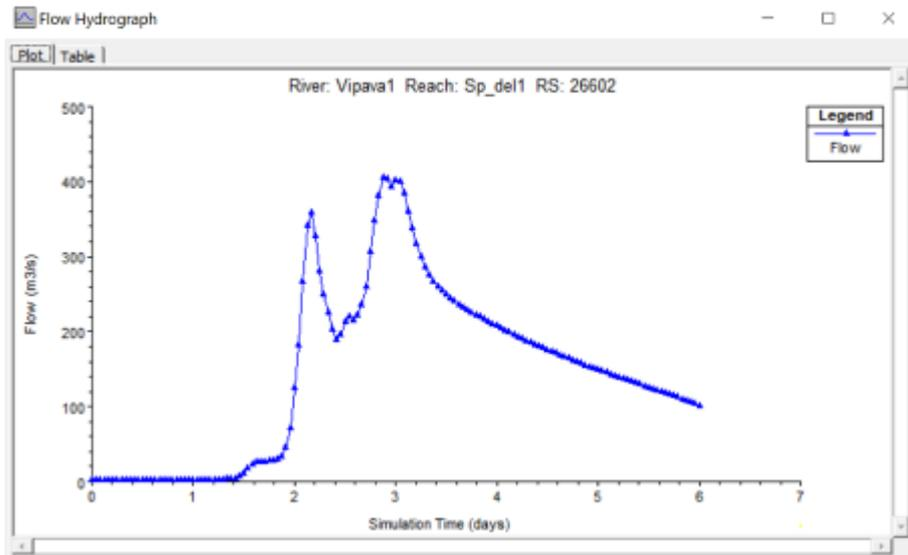
Figure 9: Hydrograph of Vipava river in Zalošče during the 2010 flood event
