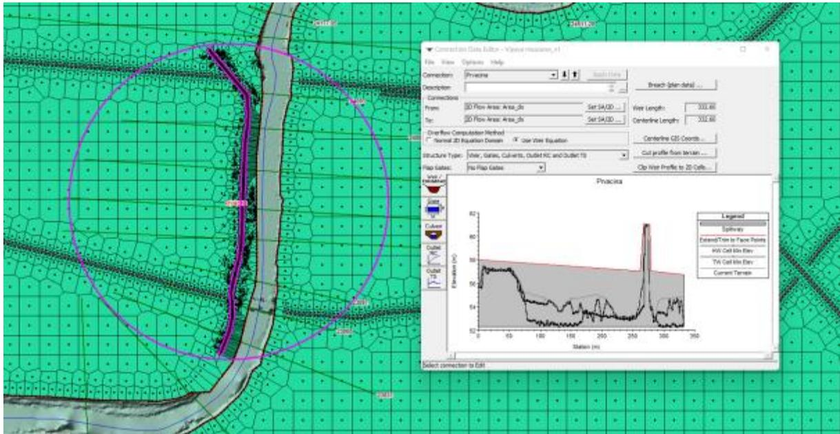
Figure 26: Implemented embankment in Pračina into the 1D-2D HEC-RAS model
