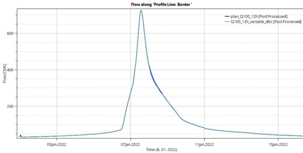
Figure 14: Hydrograph at the border profile showing results of the simulation with 12h rainfall duration input hydrographs
