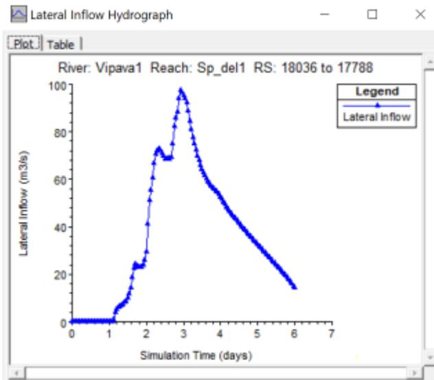
Figure 10: Lateral inflow hydrograph of Lijak (main tributary within the Vipava hydraulic model) during the 2010 flood event
