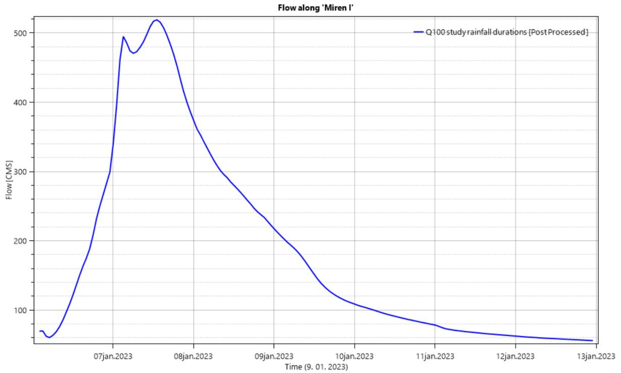
Figure 22: Results of Q100 scenario simulation with updated roughness values at gauging station Miren I
