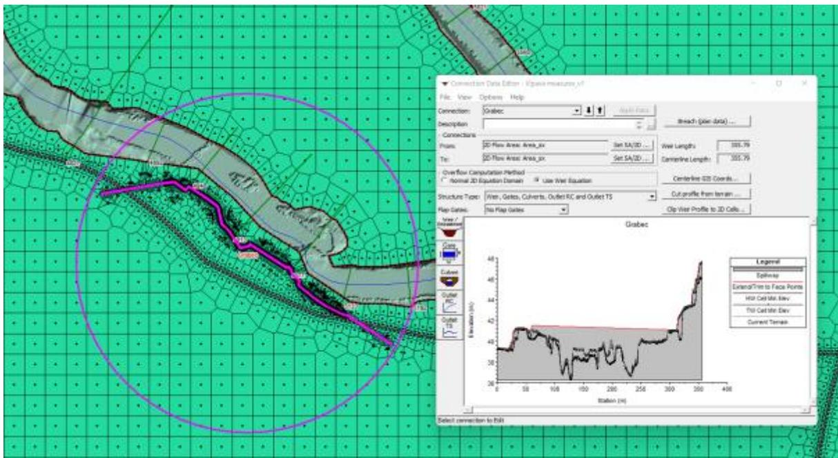
Figure 25: Implemented flood wall in Grabec-Miren into the 1D-2D HEC-RAS model of Vipava
