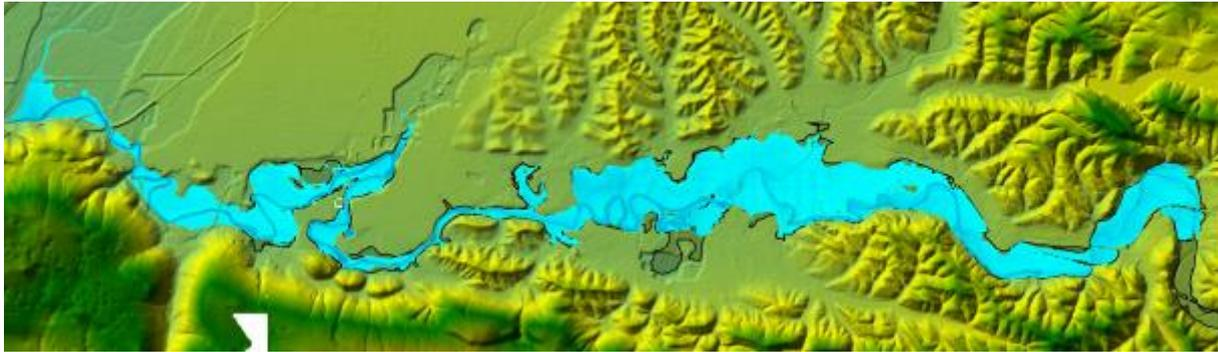
Figure 12: First calibration done by AAWA on the basis of the recorded extents of flood areas during the 2010 event
