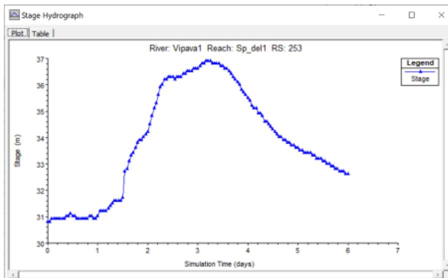
Figure 11: Stage hydrograph at Savogna d'Isonzo during 2010 flood event
