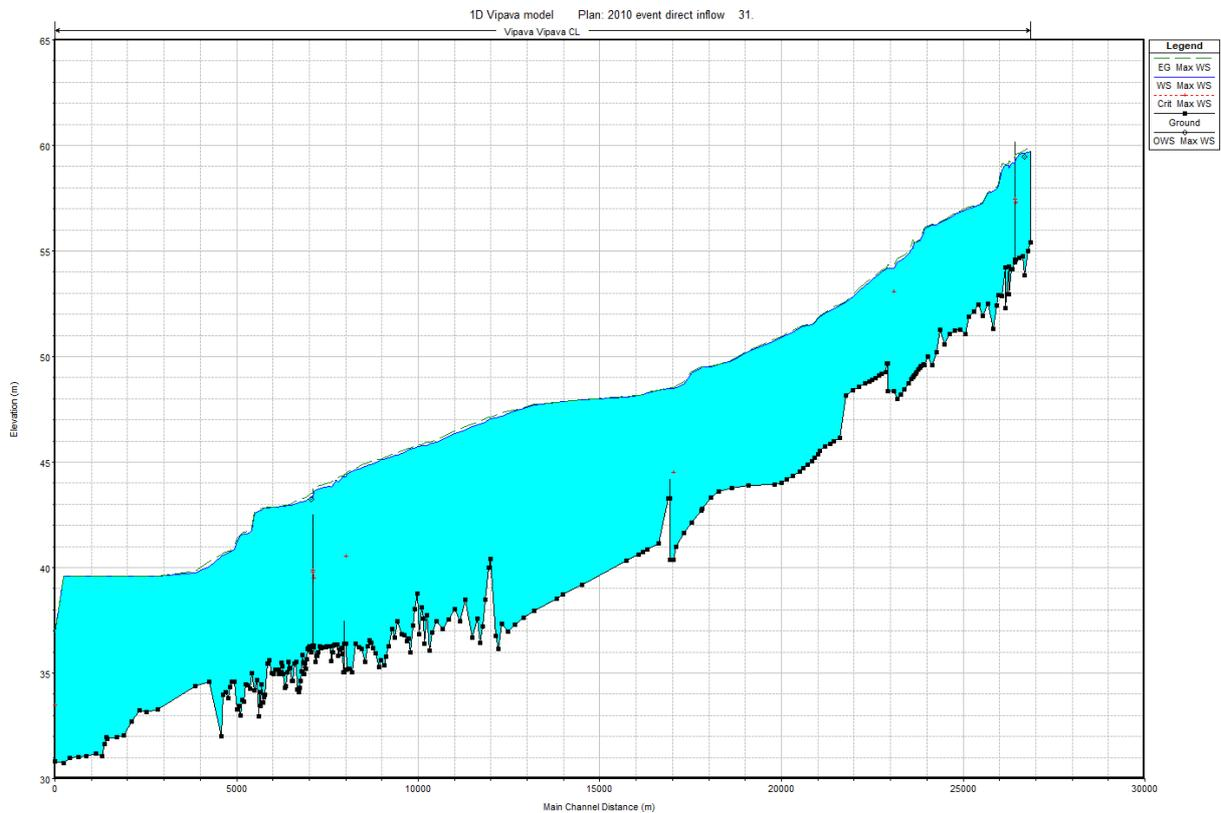
Figure 21: Profile plot with 2010 event simulation
