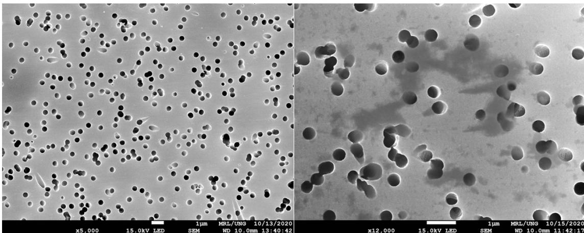
Figure 5: Scanning electron microscopy of Au coated membrane (left) before and (right) after particle deposition.
