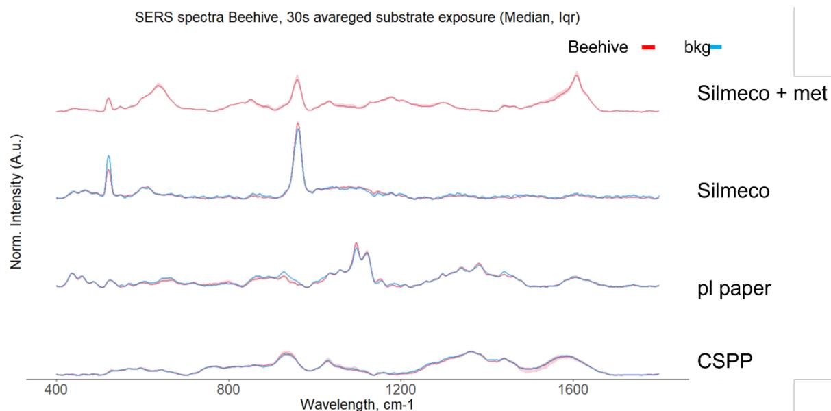
Figure 12: Over imposed SERS spectra of Beehive (red) versus background (blue), in different conditions: "CSPP" - centrifugal silver plasmonic paper; "Silmeco" - silver Silmeco substrate; "pl paper" - silver plasmonic paper; "Silmeco + met" - methanol washed beehive treated Silmeco substrate.
