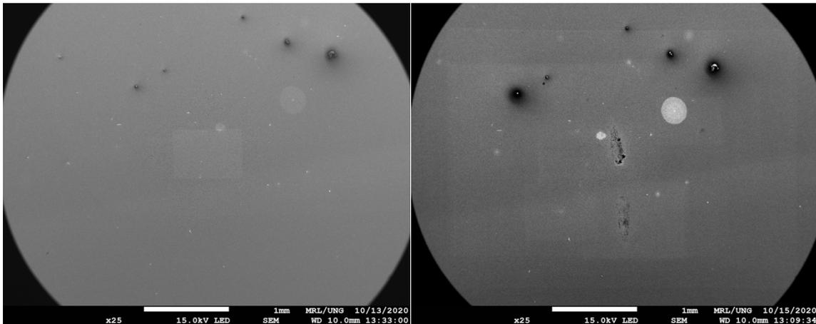
Figure 1: Scanning electron microscopy of Au coated membrane (left) before and (right) after particle deposition.
