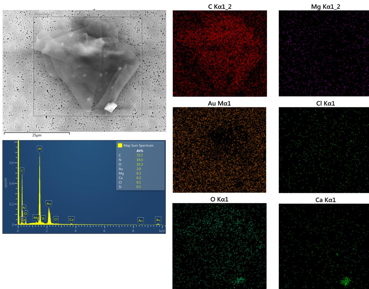
Figure 11: EDX based analysis of particles deposited on Au coated membrane. (Right) Elemental mapping of selected elements.
