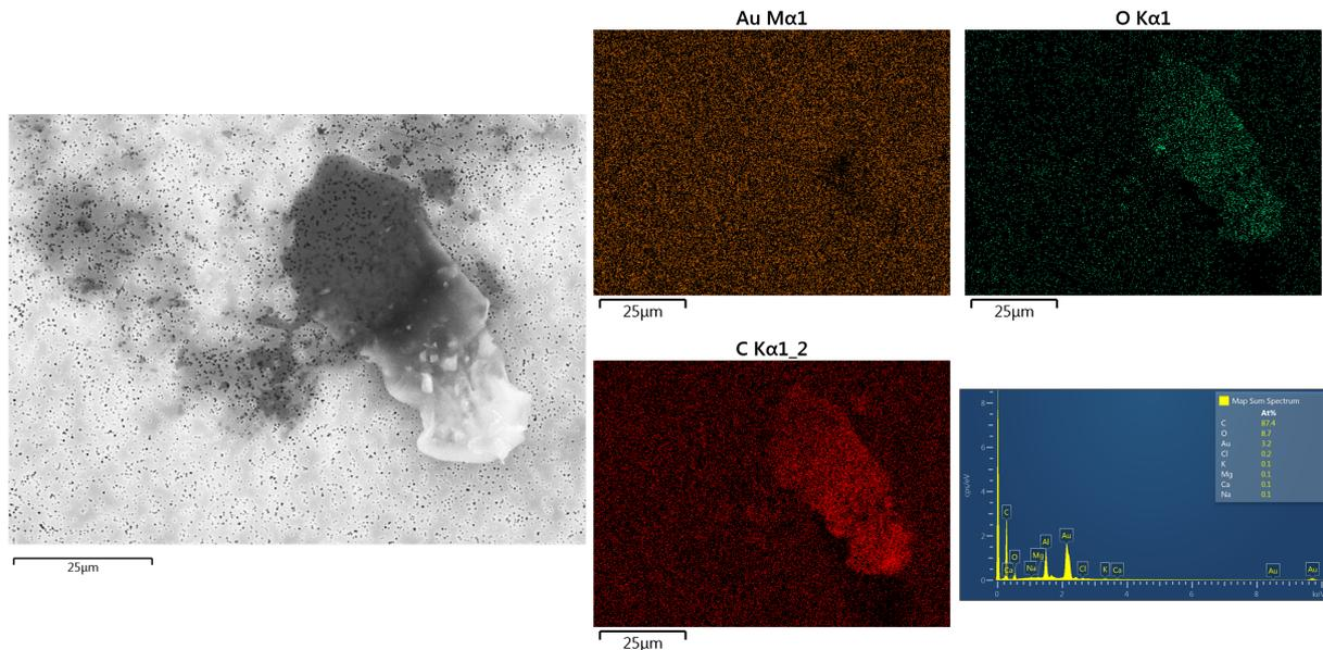
Figure 9: EDX based analysis of particles deposited on Au coated membrane. (Right) Elemental mapping of selected elements.
