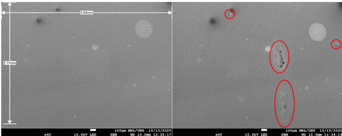
Figure 2: Scanning electron microscopy of Au coated membrane (left) before and (right) after particle deposition.
