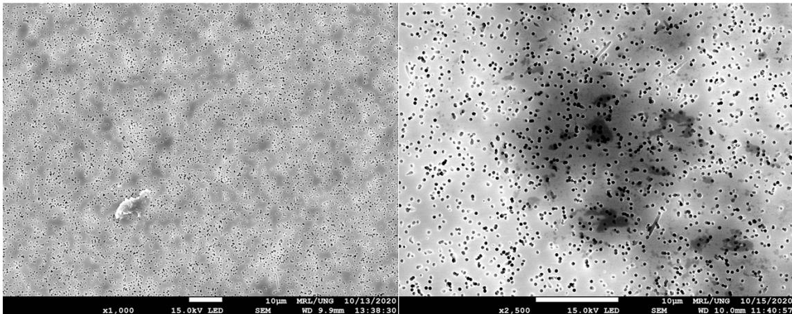
Figure 4: Scanning electron microscopy of Au coated membrane (left) before and (right) after particle deposition.
