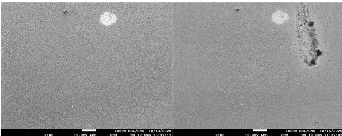
Figure 3: Scanning electron microscopy of Au coated membrane (left) before and (right) after particle deposition.
