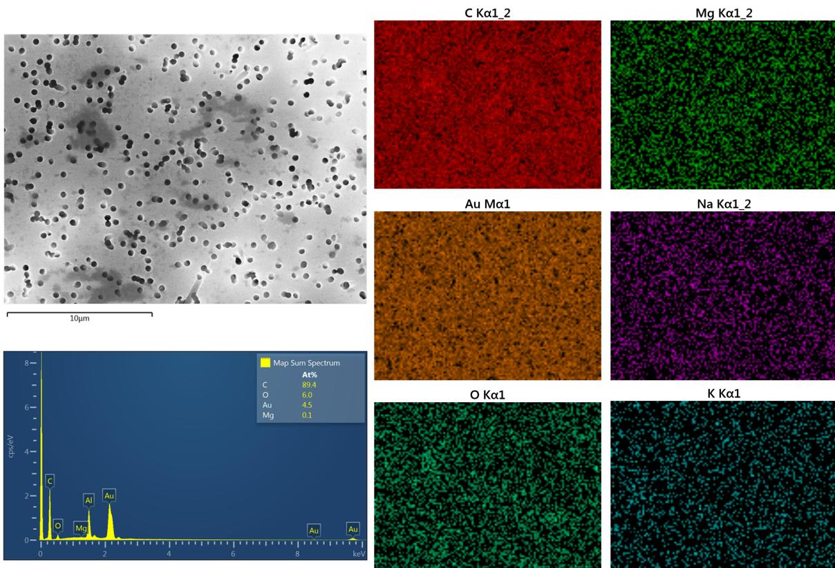
Figure 8: EDX based elemental mapping of particles deposited on Au coated membrane. Analysed region corresponds to area presented in Figure 5.
