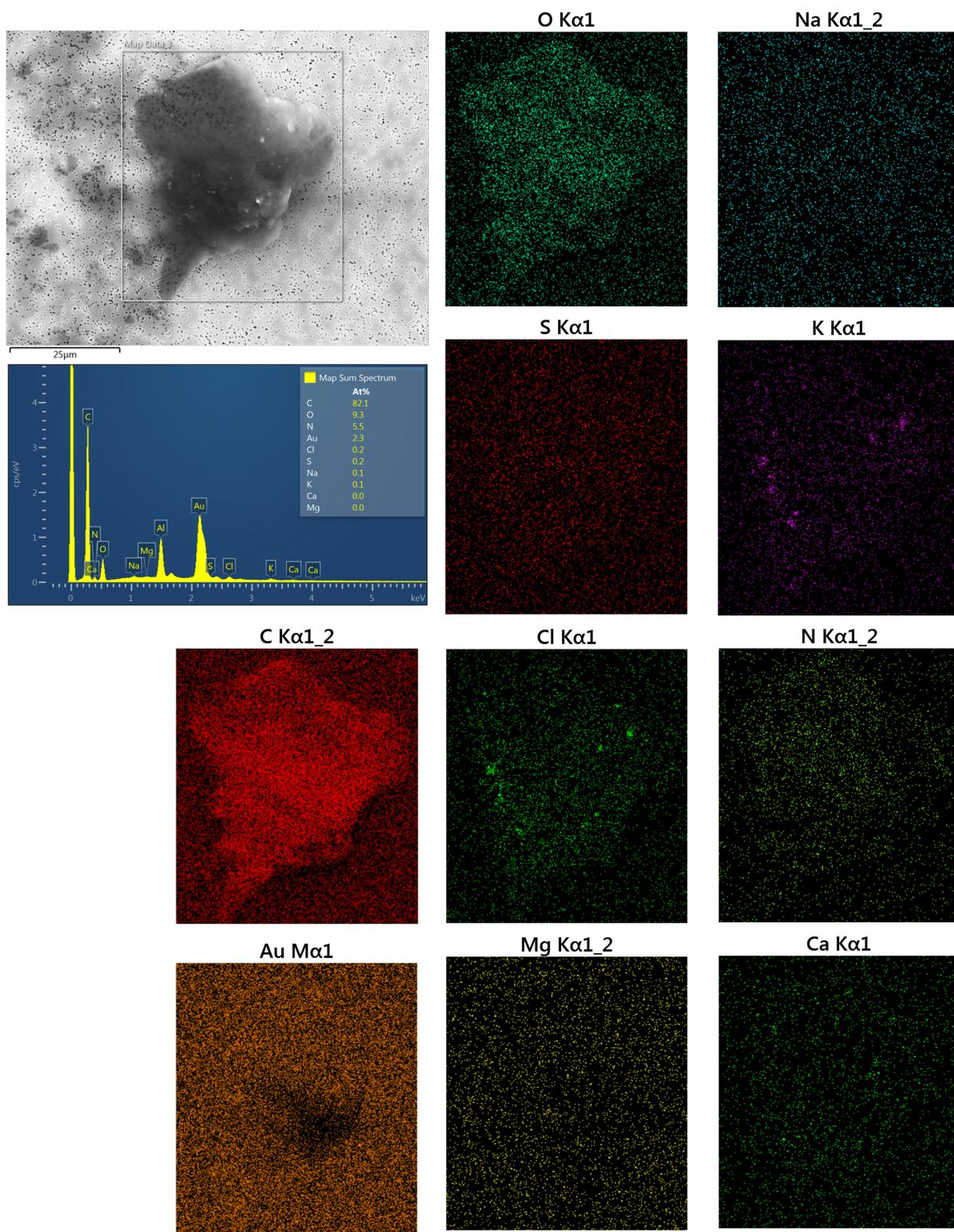
Figure 10: EDX based analysis of particles deposited on Au coated membrane. (Right) Elemental mapping of selected elements.
