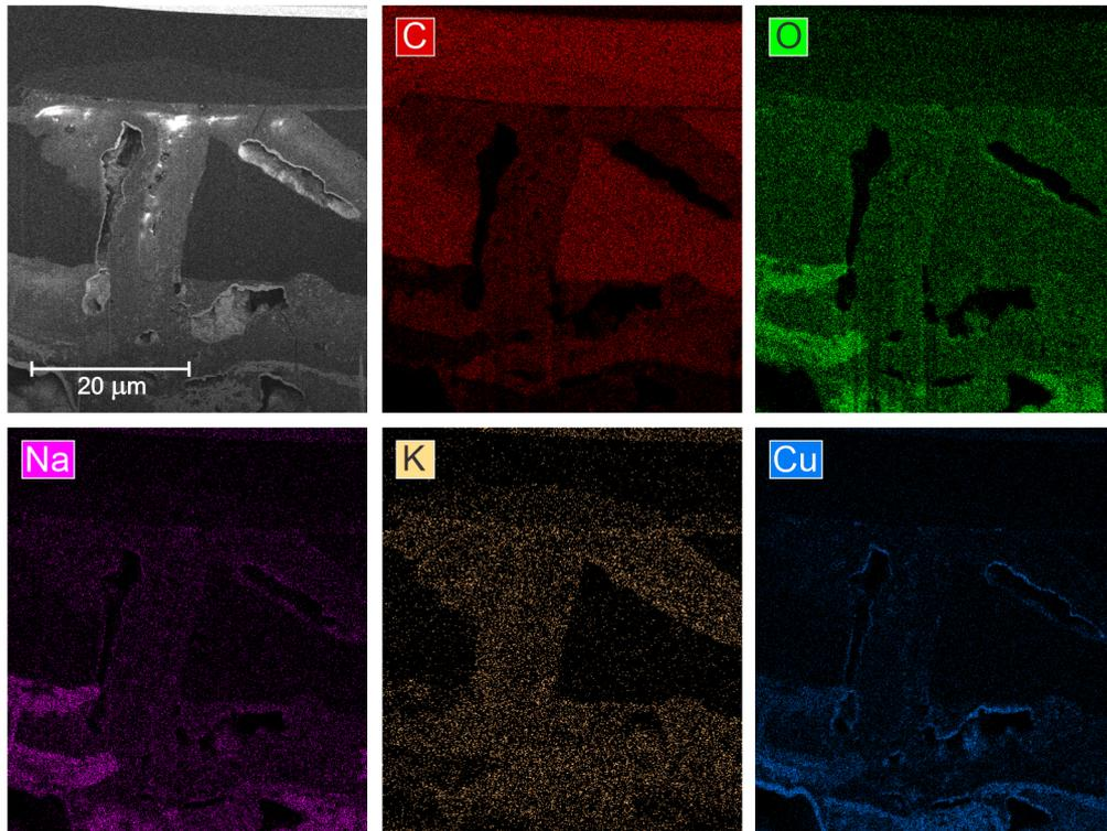
*Figure 11: EDX elemental mapping along FIB cross-section near heavily degraded region (ROI 4c) with phase contrast SEM image and corresponding EDX elemental maps (C, O, Na, K and Cu)*
