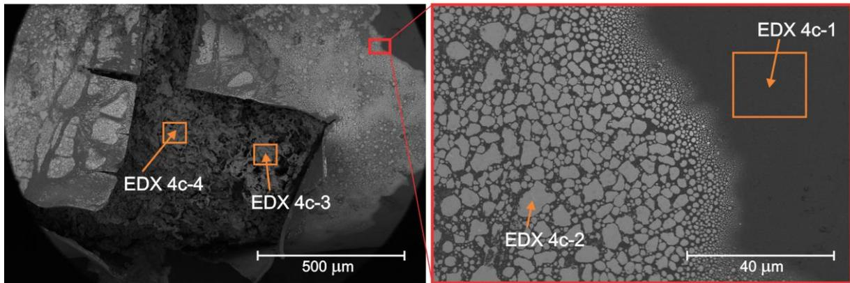
Figure 5: Phase contrast SEM images of heavily degraded region (ROI 4c) with enlarged detail (enamel surface) and denoted EDX analysis positions
