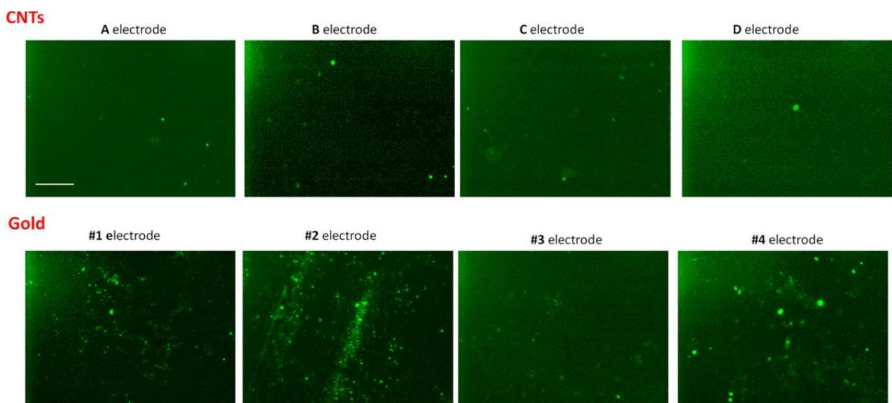
**Fig.2:** Fluorescence images of antibody bound on CNTs electrode and gold electrode acquired with a 40x objective; FITC filter. Bar 50  $\mu\text{m}$ .
