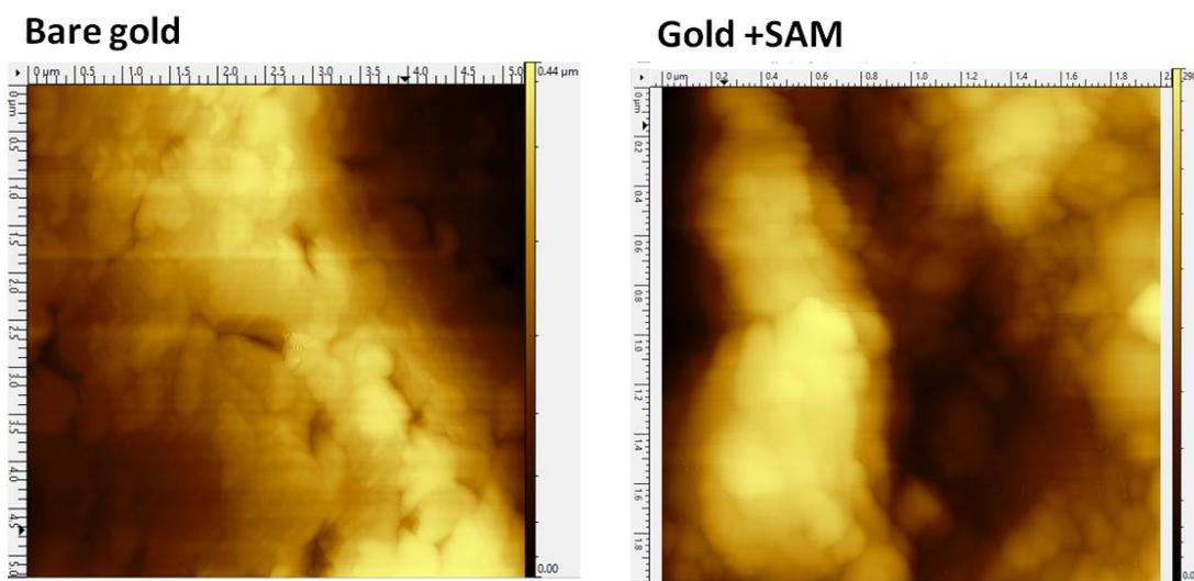
**Fig.4:** Contact mode AFM images of bare gold electrode and self-assembled monolayer of on gold electrode (cantilever Bruker MLCT K=0.02N/m).
