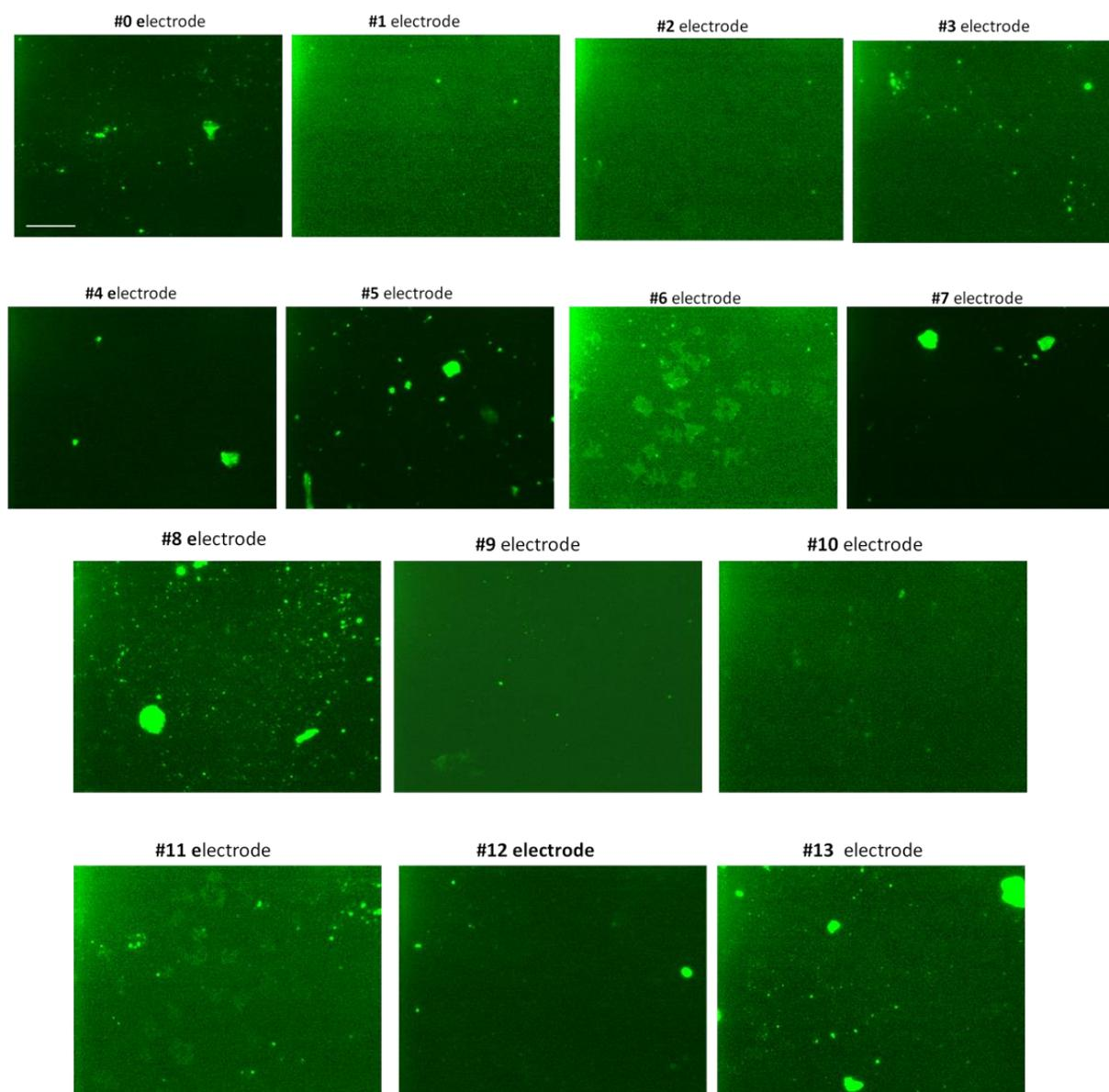
**Fig.3:** Fluorescence images of specific antibody bound to SAM functionalized gold electrodes acquired for several electrodes, 40x objective and FITC filter (Bar 50  $\mu$ m).
