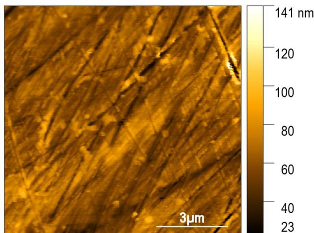
**Fig.5:** Contact mode AFM images of pure flat gold electrode (cantilever Nanosensors ATEC –FM-20 K=0.7-9 N/m)).
