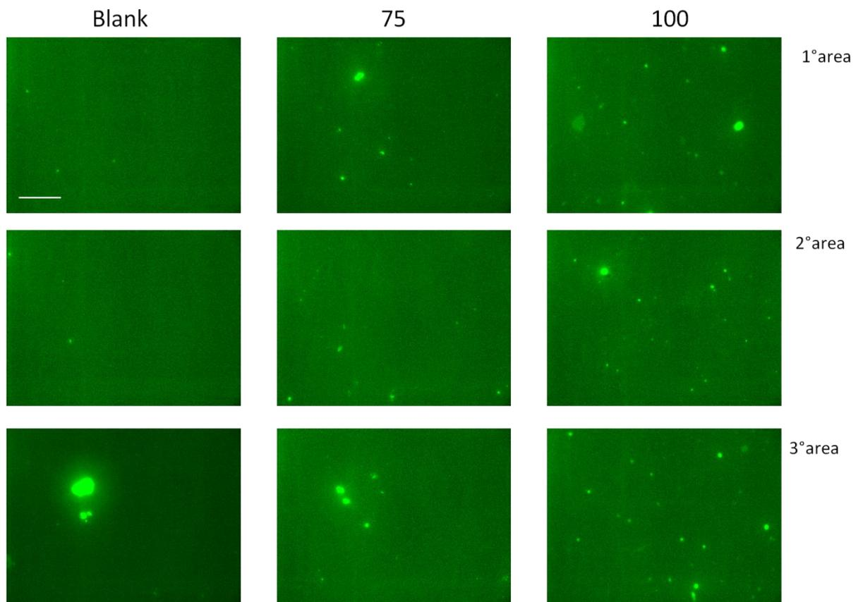
**Fig.1:** Fluorescence images of specific antibody bound on CNTs electrode acquired with a 40x objective; FITC filter. Blank is bare CNTs in absence of antibody, 75 and 100 are different concentration of antibody. Images were acquired on 3 different areas for each samples (Bar 50  $\mu\text{m}$ )
