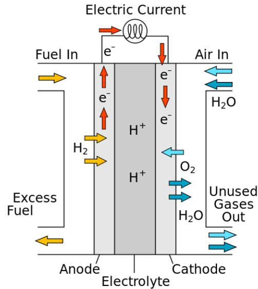
Figure 1 Schematics of hydrogen fuel cell
