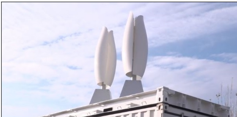
Figure 2.1 Two small wind turbines placed on a sea container at WSV Haringvliet (Hellevoetsluis), (Troelstra,2021)
