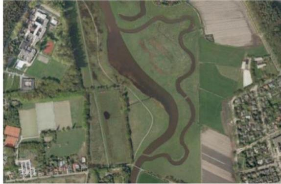
*Figure 2: The channelized and normalised Mark River and the (artificial) Oudhof Meander at the vicinity of Ulvenhout Village (photo: Waterschap Brabantse Delta)*
