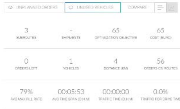
Figure 3.20: Southend Temple Farm, results for fortnightly collections with triple waste volume and two containers at the mini-hub
