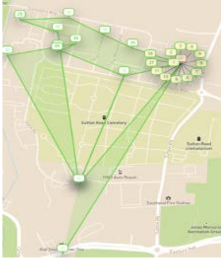
Figure 3.39: Southend Temple Farm, possible route for monthly collections with triple volume and two containers at the depot
