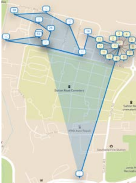
Figure 3.25: Southend Temple Farm, possible route for monthly collections with triple waste volume and two containers at the mini-hub
