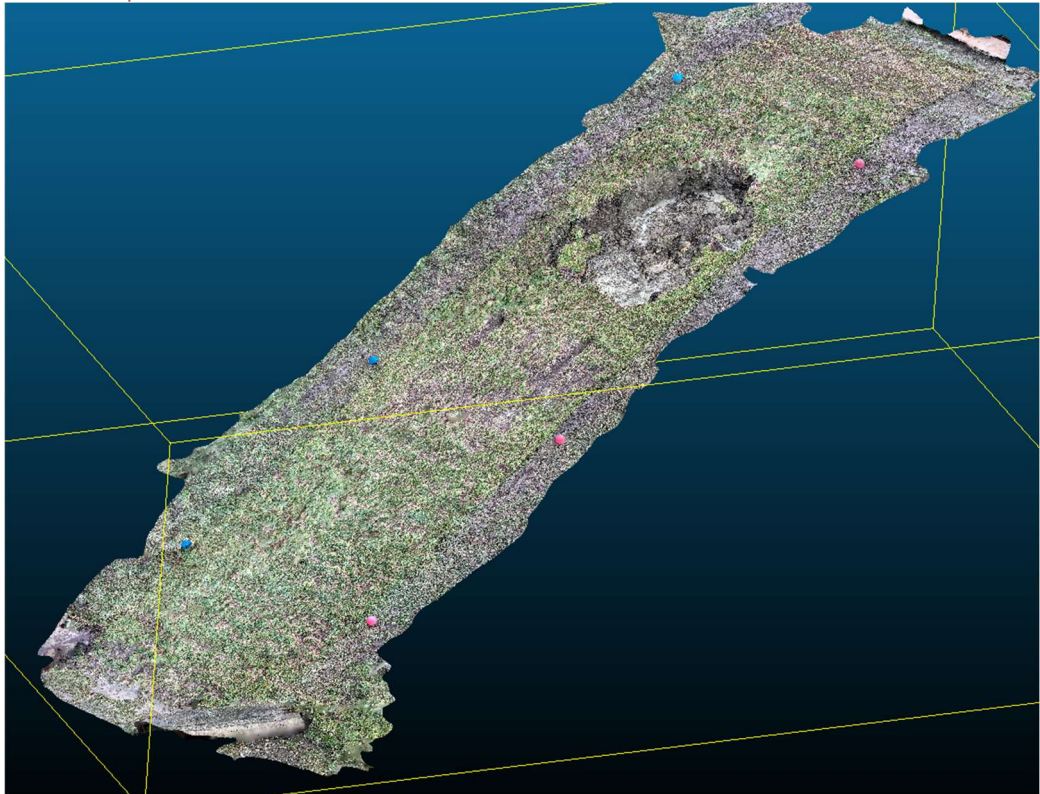
Figure 10: 3D view of the Handheld Lidar point cloud data of a damaged section.
