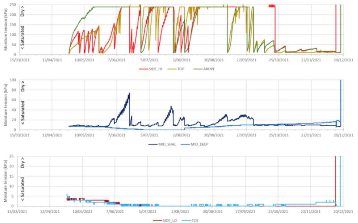
Figure 25: Soil moisture evolution in 7 measurement points at N-OF10 test site.
