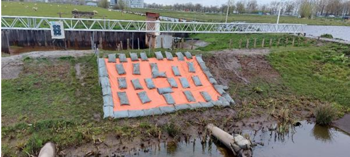
Figure 21 Three-dimensional water inflow experiment at intermediate scale, Flood Proof Holland, TU Delft, spring 2022
