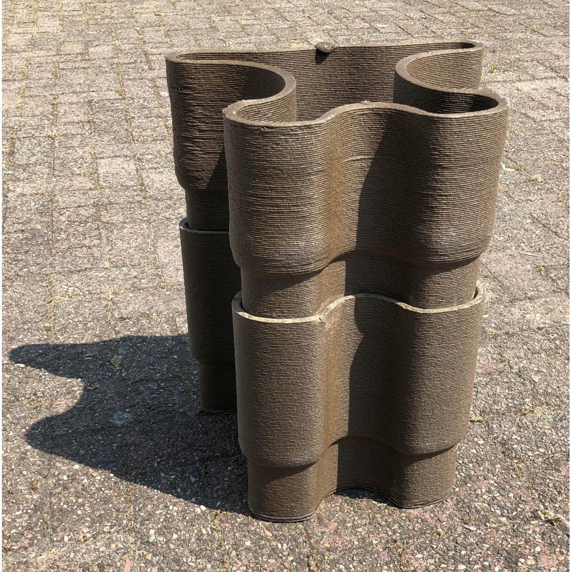
Figure 14 Fitting of two prototype fender profiles of TPS-NF.
