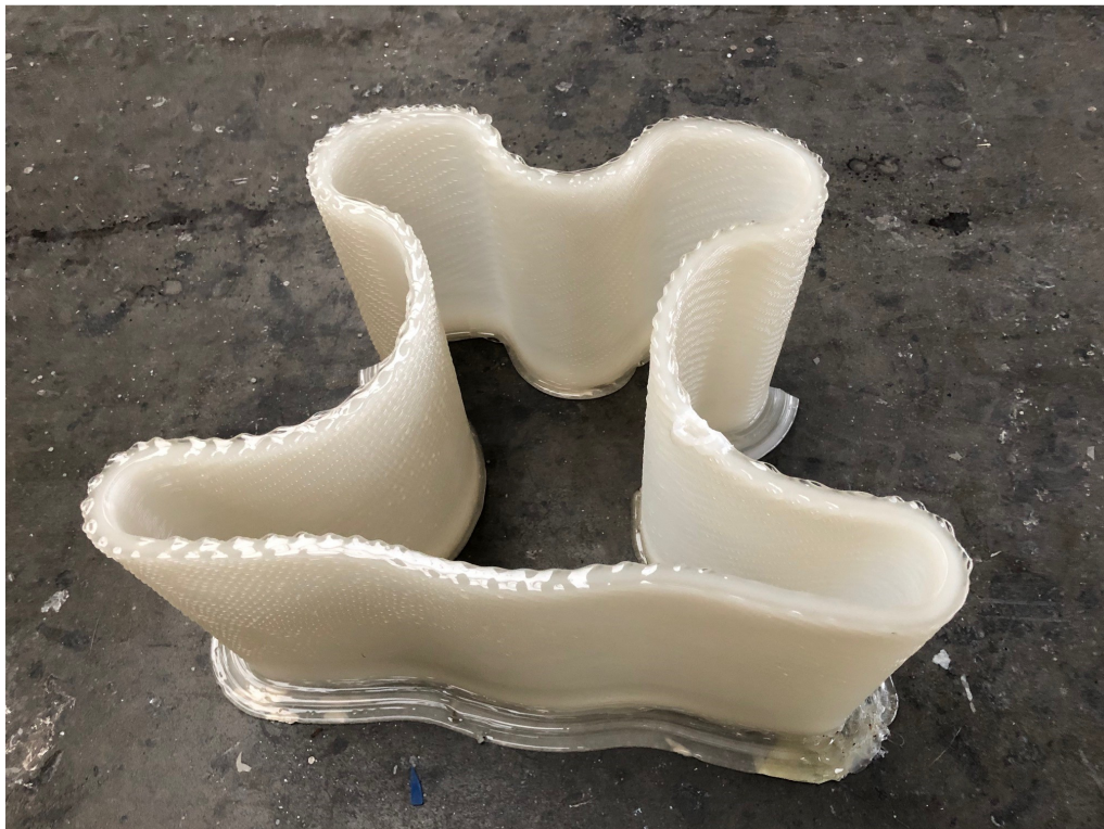
Figure 10 Further improved fender profile (3) printed with PLA.
