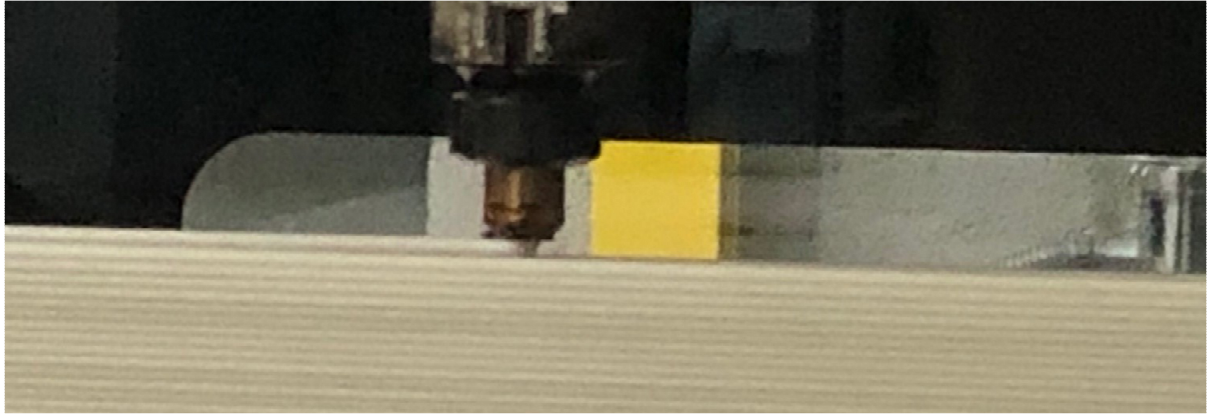
Figure 4 Detail of the formation of the layer by the nozzle.
