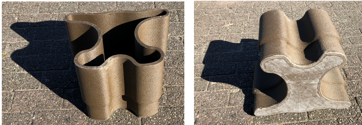
Figure 14 Printed prototype fender profile made of TPS-NF.
