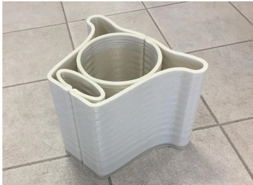
Figure 7 Improved fender profile design, printed in rPETG-GF30.
