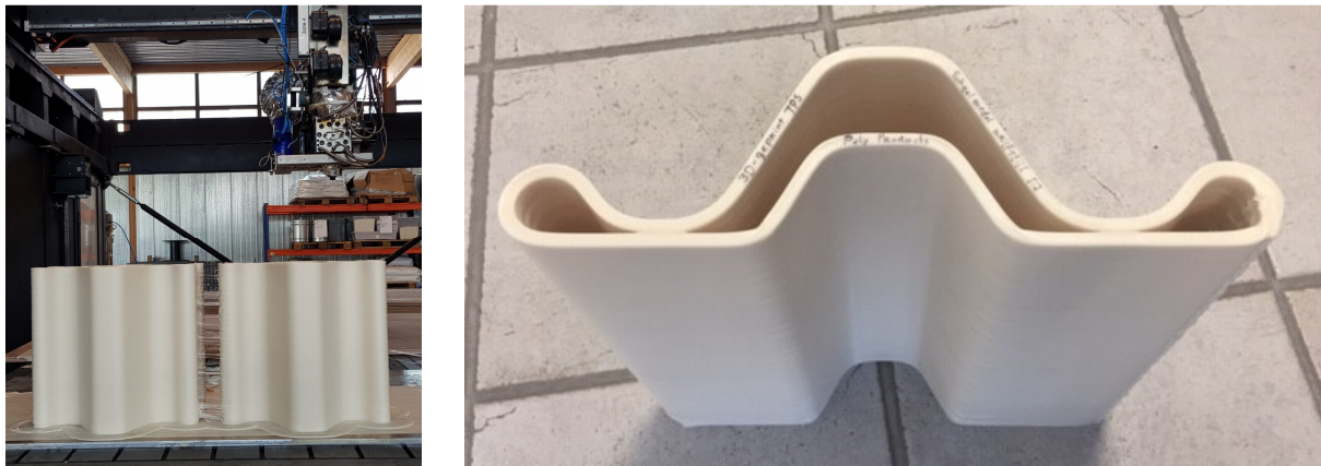
Figure 6 Printing of four prototype fender scale products and cross-section.
