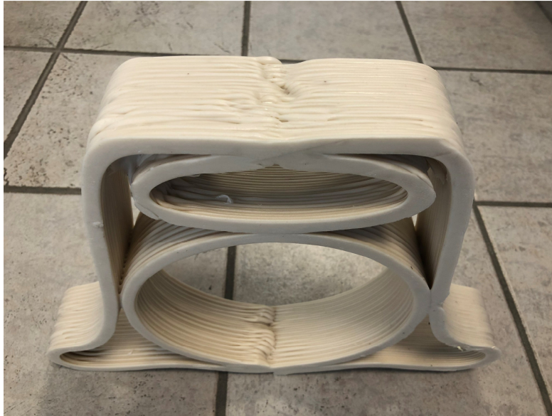
Figure 8 Improved fender profile (10 mm wall-thickness) printed in TPS.
