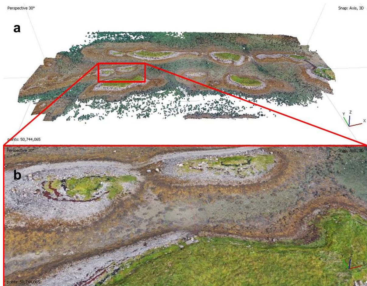
Figure 15: Example dense point cloud from mid-tide, 120 m survey of site 2 (a) and a close up of the section highlighted in red (b).
