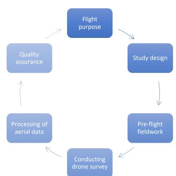
Figure 1: Activities involved in UAS-based mapping, adapted from Tmušić et al. (2020)
