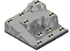
Figure 8: Example of well-placed GCPs (Propeller Aero, 2018)
