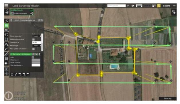
Figure 4: Example of plan flight route showcasing the flight pathway (UgCs, n.d.)
