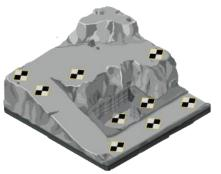
Figure 7: Example of 'badly' used GCPs (Propeller Aero, 2018)
