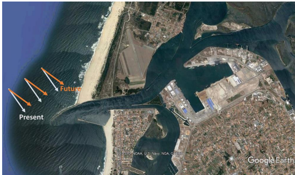
Figure 3: Hypothetical example of change in wave direction with respect to coastal ports structures
