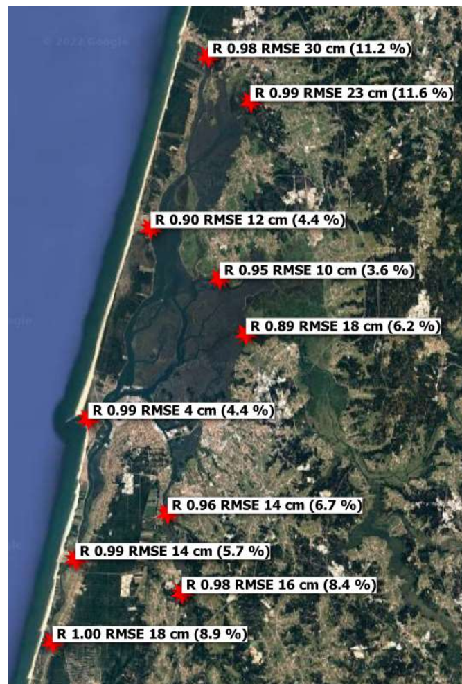
Figure 4 – RMSE and correlation of the hydrodynamic model tide levels in 10 stations for a one month simulation (July 2019).
