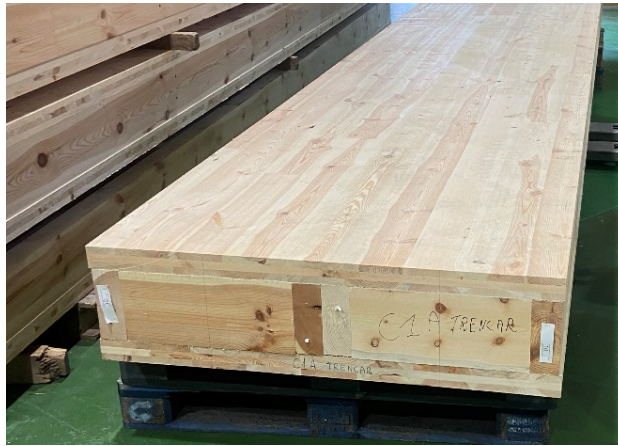
Figure 2. Manufactured full size C panel
