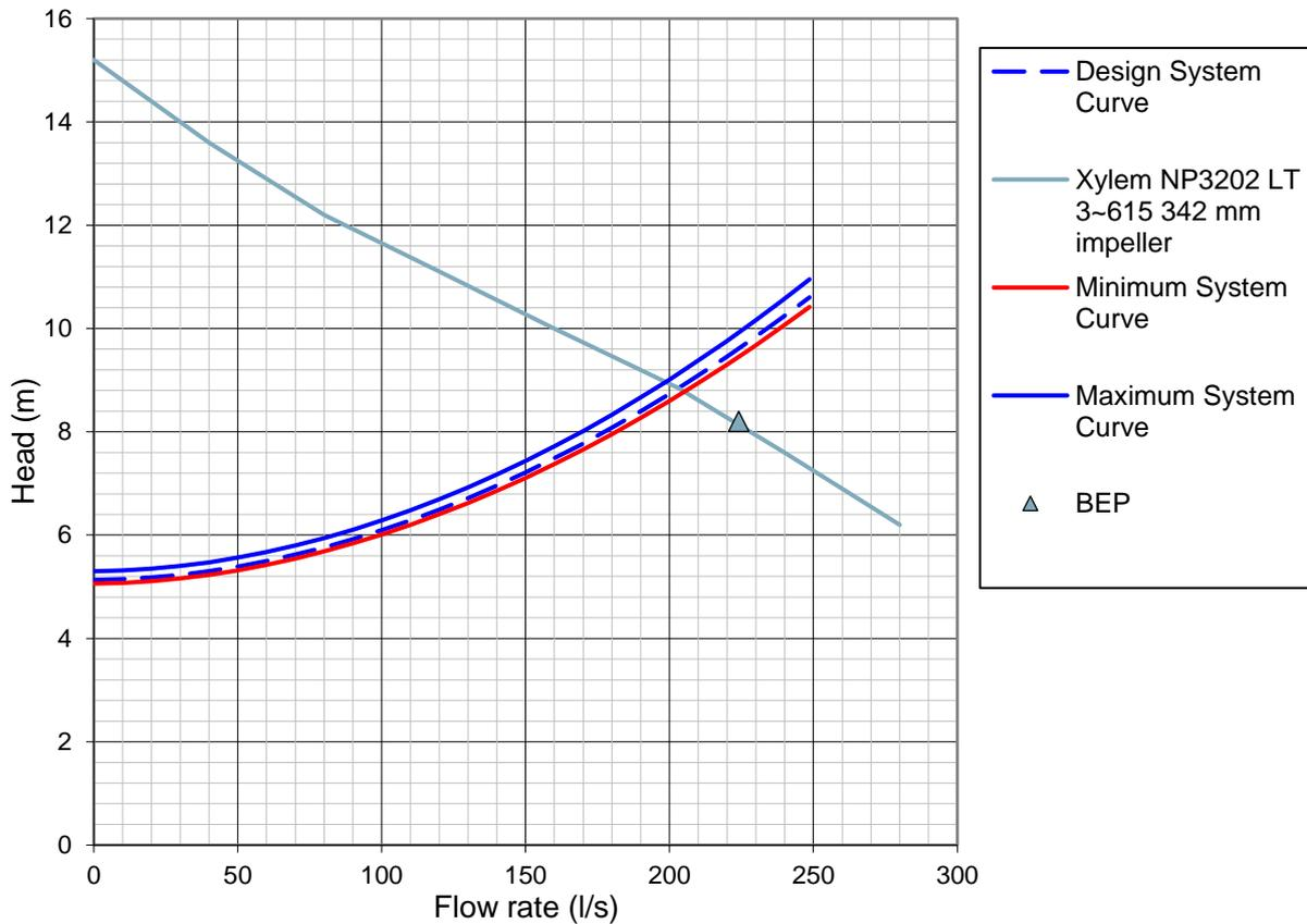
Figure 9 - Alternative pump selection, Xylem (single pump, duty operation)
