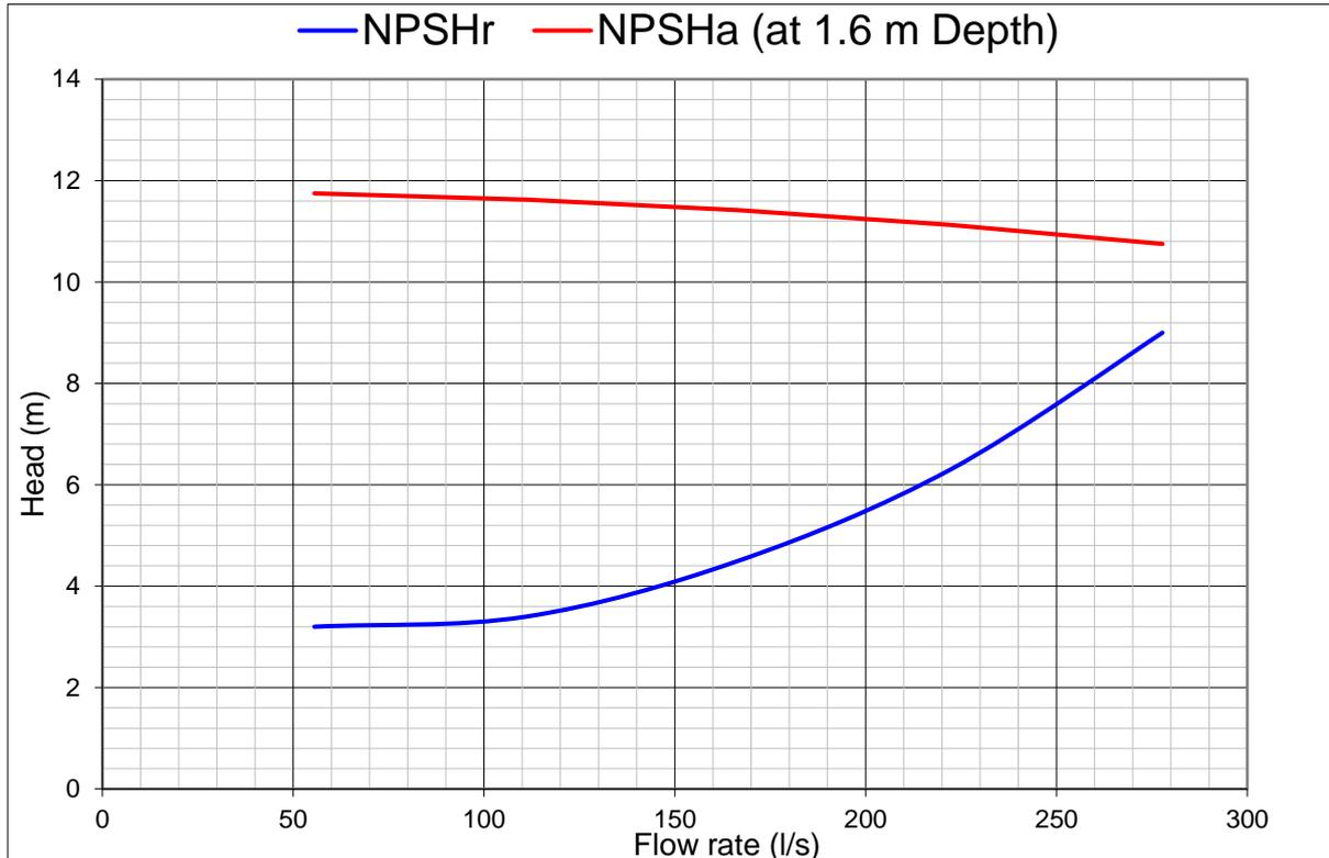
Figure 4 – NPSH Curves for KSB KRTK 200-330/414 UG pump
