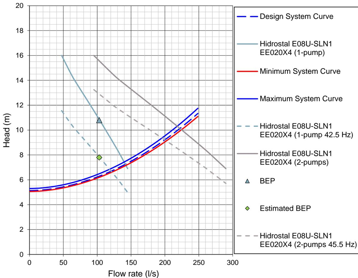
Figure 8 – Alternative pump selection, Hidrostal (two pump duty/assist operation)
