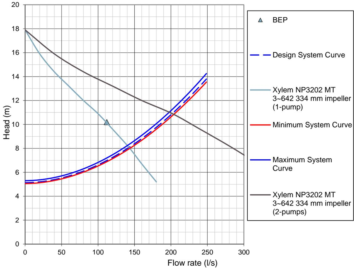
Figure 10 – Alternative pump selection, Xylem (two pump, duty/assist operation)
