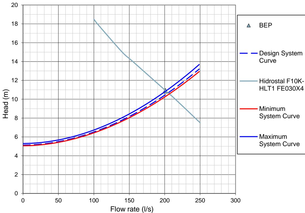
Figure 7 – Alternative pump selection, Hidrostal (single pump, duty operation)
