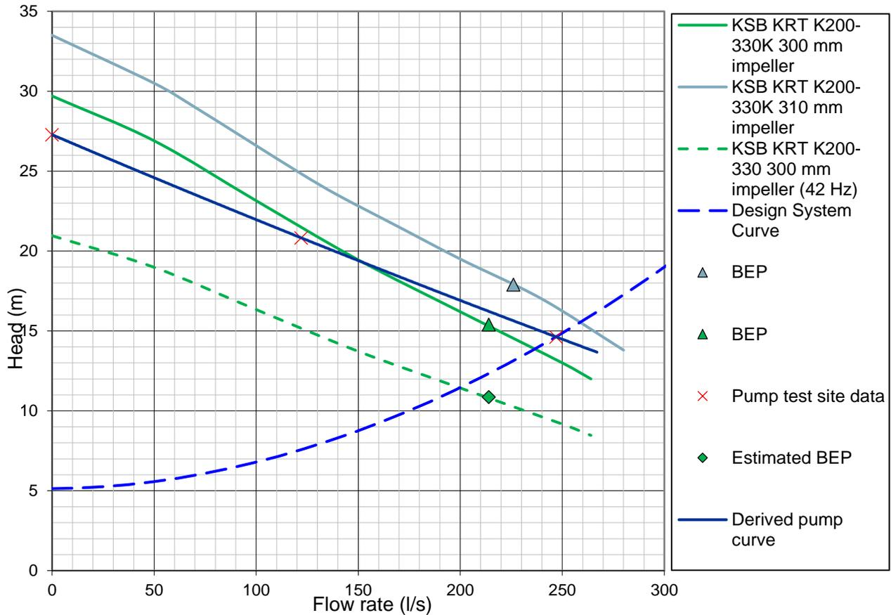
Figure 3 – Derived System Curve for Calcutt PS
