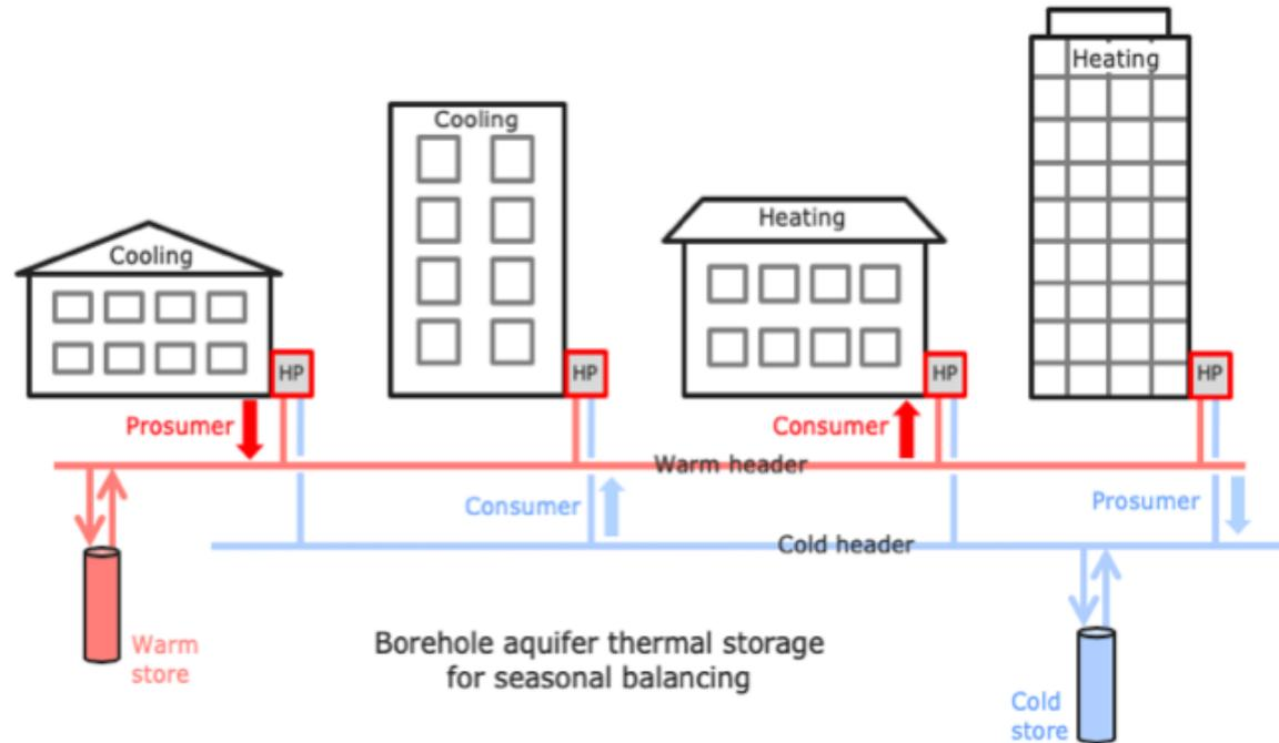
**5DHC schemes allows flexibility in terms of temperature and timing for building connections – a 'plug and play' approach.**
