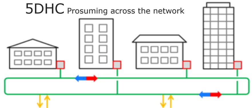
It is clear from that there is a progression/transition path from 3DHC to 4DHC due to the similar system architectures (topologies) involved. However, whilst 5DHC appears to be the next logical step, it has quite different shape, structure and approach. For discussion purposes, we have retained the term 5th generation (5DHC) but it should probably be viewed as an entirely different type of DHC altogether.
