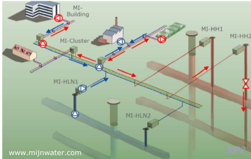
The Minewater project in Heerlen, Netherlands is a working 5<sup>th</sup> generation DHC scheme. The scheme uses decentralised heat pumps and is based around mine water from a warm mine and a cold mine with a spine (backbone) as shown opposite.
