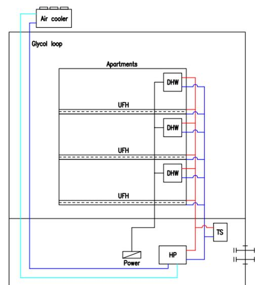
SH: Heat pump, 45–35°C with underfloor heating
