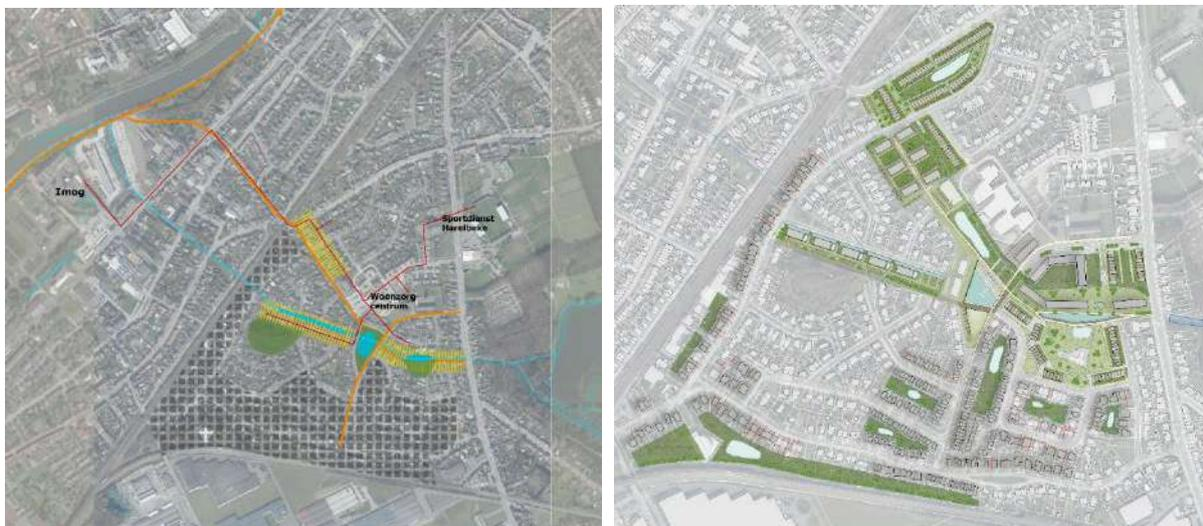
Figure 58: introducing a district heating network in the 'Collegewijk' in Harelbeke, it passes through the neighbourhood and connects the waste incineration plant IMOG with a health care centre and the sport facilities of the municipality. Figure 59: the district heating network stimulates densification of the neighbourhood.
