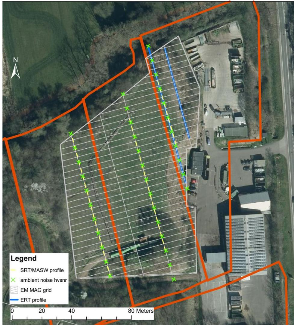
*Figure 2: Planned measurement layout on investigation area 1*
