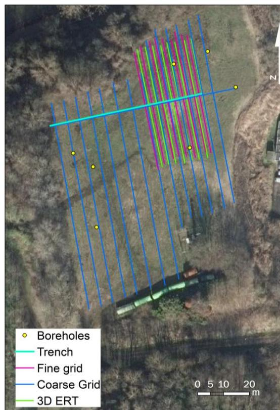
*Figure 4: Planned geophysical survey. The EM acquisition is formed by a fine and coarse grid displayed in pink and blue respectively. The green grid represents the location of the 3D ERT acquisition. Yellow dots represent the boreholes and the blue line the planned trench (and the high-resolution ERT/IP profile).*
