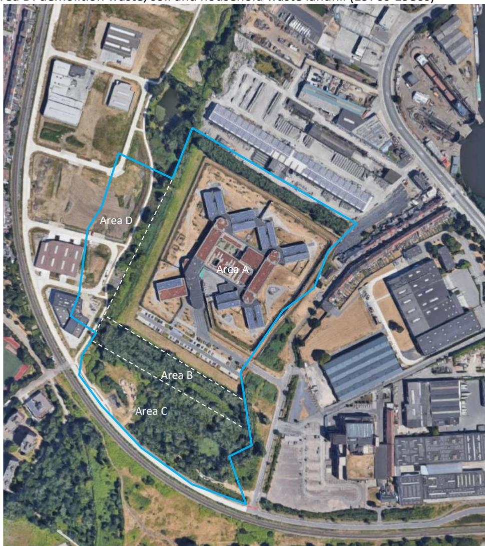
*Figure 10 - Aerial photograph 2020 with the location of the Landfill n°2211 and its geographical division based on type of waste deposits.*
