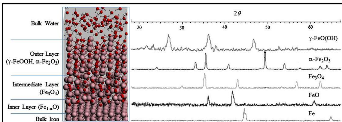
Figure 22: Passive layer components (Pan et al 2011)
