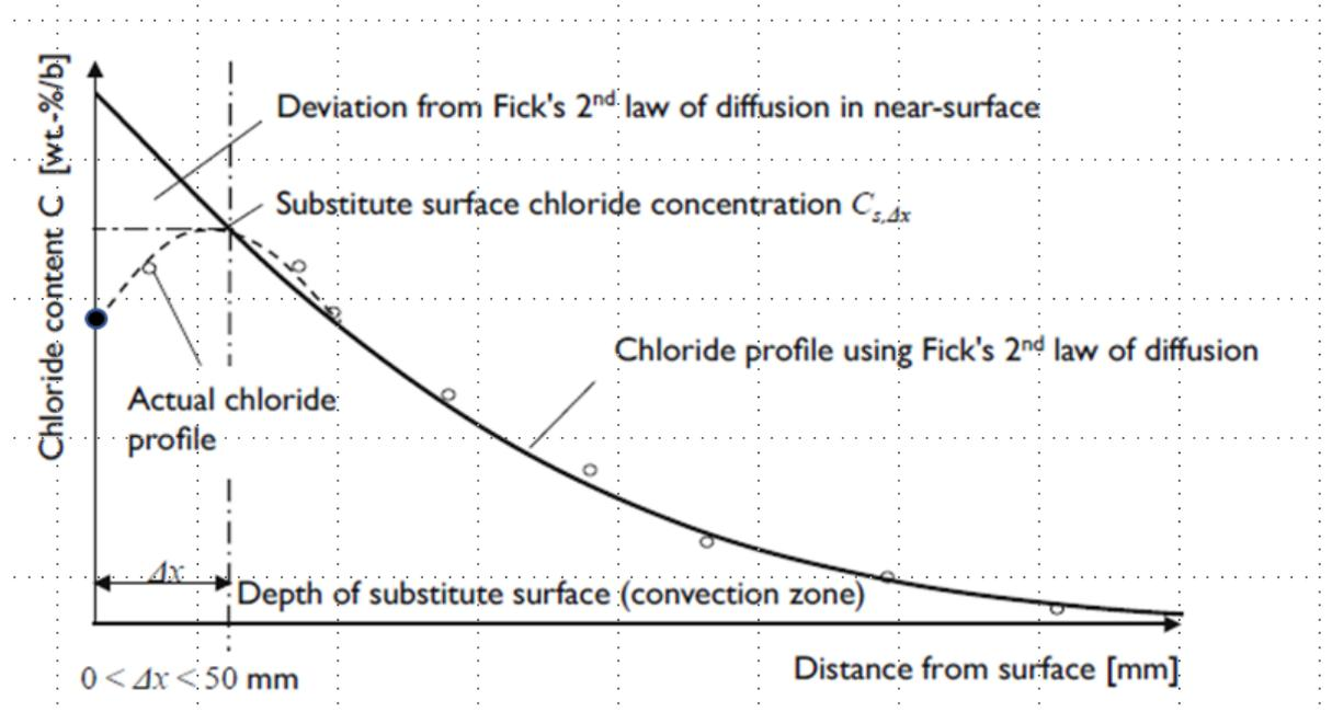
Figure 20: Near-surface deviation of chloride profiles from Fick's law of diffusion in the convection zone
