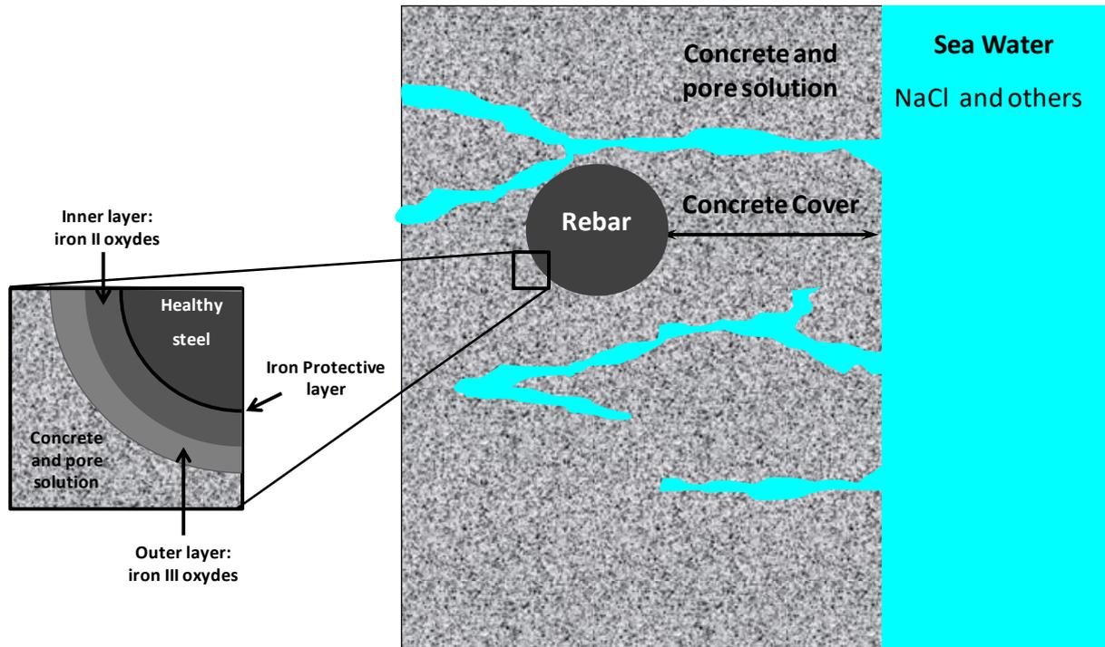
Figure 21: Reinforced concrete exposed to seawater and schematic protective layer on steel reinforcement as a two-layered structure [Soive 2021].
