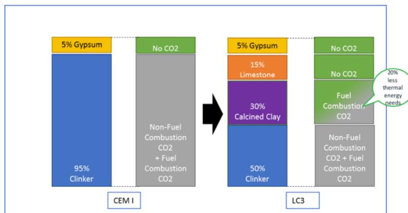
Figure 25: Composition and CO<sub>2</sub> savings between an ordinary Portland cement and a LC<sup>3</sup> (source: <https://lc3.ch/why-lc3>)
