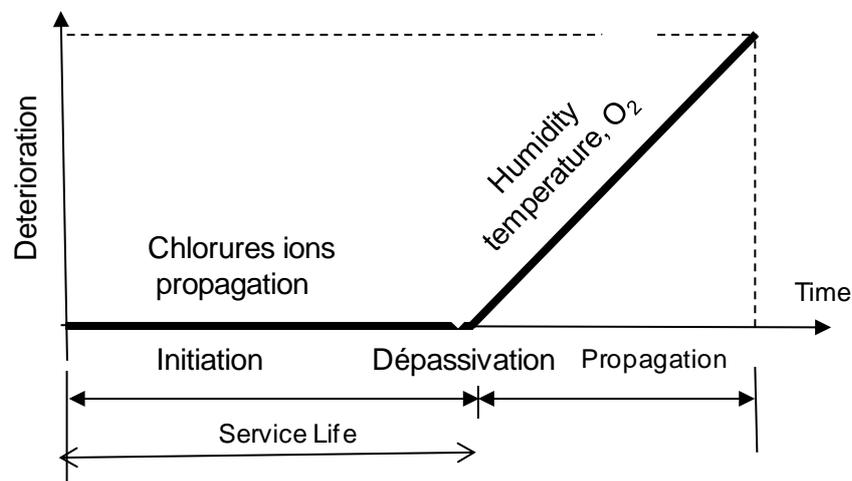
Figure 17: Diagram inspired from Tuutti diagram [Tuutti 1982]
