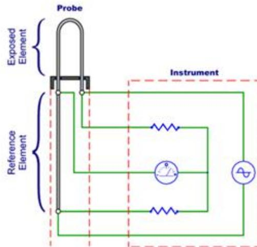
Figure 1: Schematics of a possible execution of an ER-probe. (<http://www.alspi.com/erintro.htm>)
