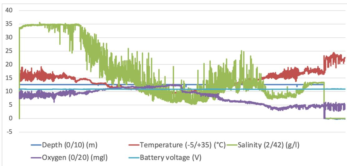
Figure 4: Deviations of parameters (salinity) measured by a multisensory probe after 7 months without maintenance. © F. Schoefs-Université/Capacités.
