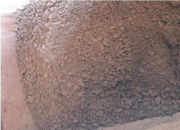
**Figure 3.1.11: SSA residues produced by TetraPhos® process (Picture: REMONDIS Aqua Industrie GmbH & Co.KG./P. Herr)**
