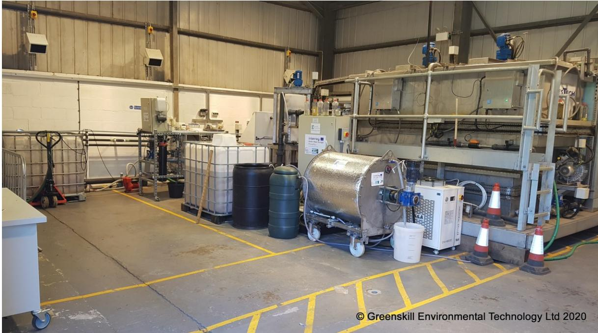
Figure 4.1.9: Greenskill Environmental Technology Ltd. 75L and 500L PBRs installed at the Wastewater Development Centre in Bo'ness (Picture: Greenskill Environmental Technology Ltd.)
