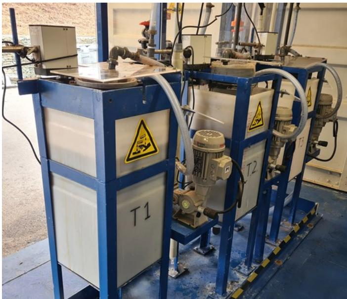
**Figure 3.4.24 Tanks used for leaching and precipitation in I3 demonstrator (Picture: ULiège/Z. Shariff)**
