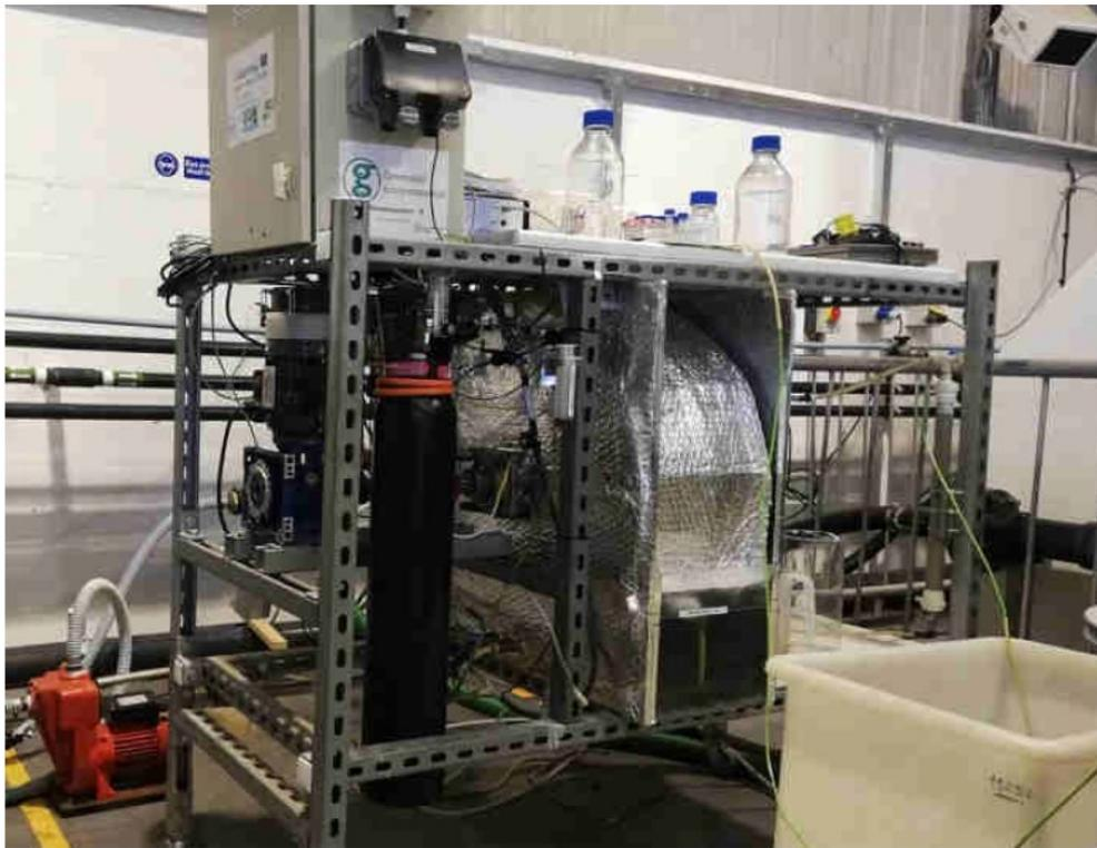
Figure 4.1.10: Greenskill Environmental Technology Ltd. 75L PBR implemented at the Wastewater Development Centre in Bo'ness (Picture: GCU)
