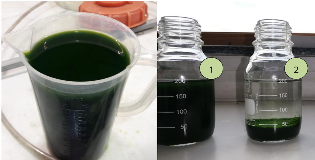
**Figure 4.1.16: On the left, microalgae biomass concentration in the PBR. On the right, microalgae biomass sedimentation after 5 min without (1) and after the addition of  $0.5\text{g L}^{-1}$  of NaOH (2) (Picture: GCU)**
