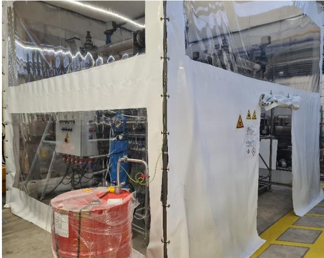
**Figure 3.4.22: Mixer-settler equipment for solvent extraction. Installed inside the Chemical Engineering Hall of ULiège (Picture: ULiège/Z. Shariff)**
