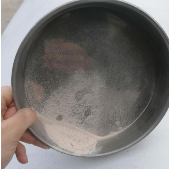
**Figure 4.3.13: Recovered P product from the pilot plant at the WWTP (Picture: MTU)**
