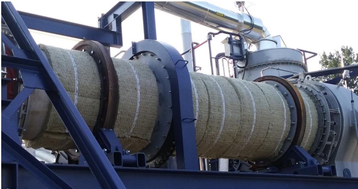
Figure 3.2.8: External isolation (Picture: Emschergenossenschaft/L. Pamuk)
