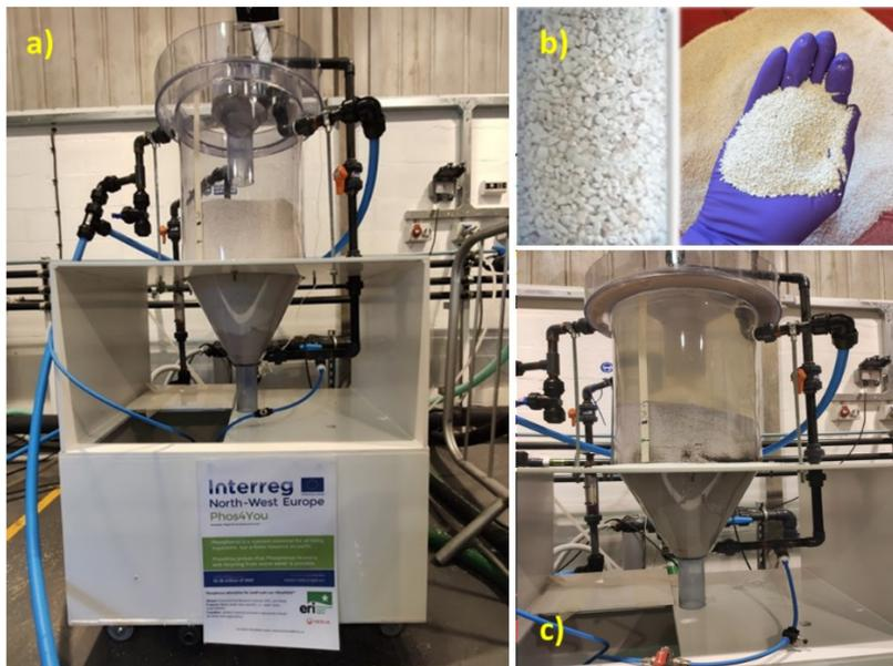
**Figure 4.2.7: FILTRAFLO™-P pilot reactor designed by Veolia (a), the CCM adsorbent developed by ERI (b) and the airlift supported self-backwashing system visible at the bottom and right side of the unit (c) (Picture: ERI)**
