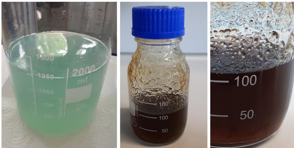
**Figure 3.1.22: Phosphoric acid samples after evaporation (left: without Al-separation, right: after Al-separation) (PARFORCE Engineering & Consulting GmbH 2021)**
