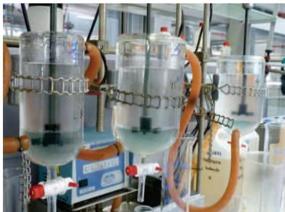
**Figure 3.1.14: Experimental set up for Solvent extraction stage (Fe-extraction) (Picture: Técnicas Reunidas)**
