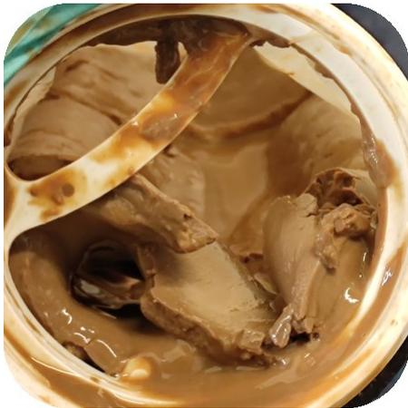
Figure 3.4.31: Filter bag containing the filter cake (Picture: ULiège/Z.Shariff)
