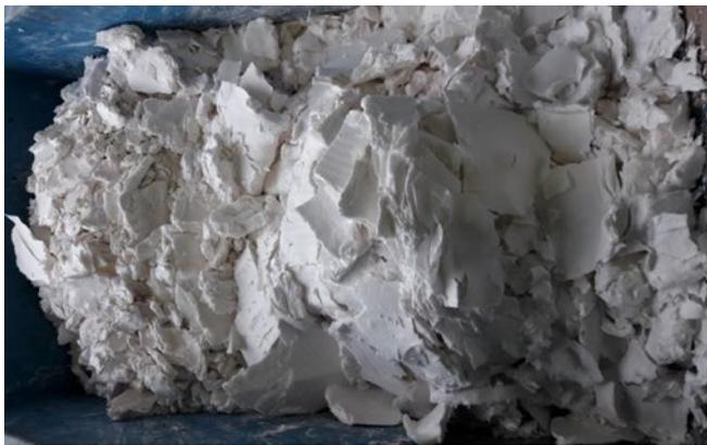
**Figure 3.1.9: Synthetic gypsum produced by TetraPhos® process (crystallisation/separation step)**
