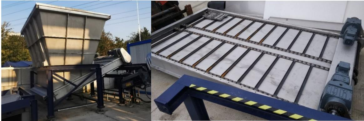
Figure 3.2.4 a and b: Drag chain conveyor (Pictures: Emschergenossenschaft/L. Pamuk)
