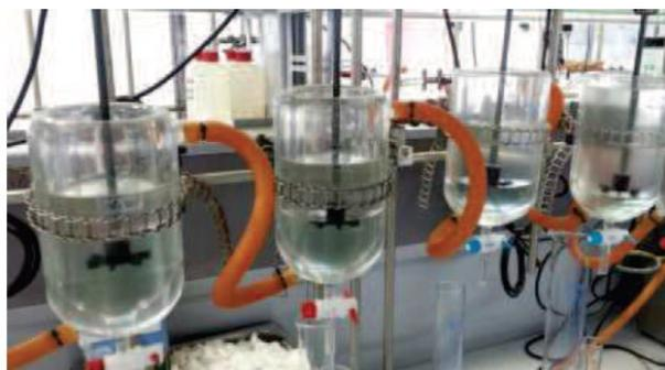
**Figure 3.1.15: Experimental set up for Solvent extraction stage ( $H_3PO_4$ -extraction) (Picture: Técnicas Reunidas)**
