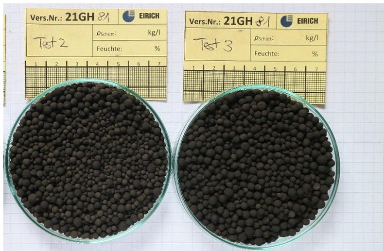
**Figure 3.2.15: Pellets of EuPhoRe<sup>®</sup>-SSA and 2 different types of salt-solution LCA for I1**
