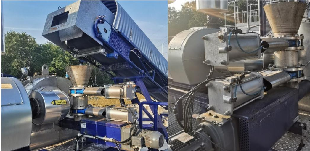
Figure 3.2.6 a and b: Dosing of additives and air lock (Pictures: Emschergenossenschaft/L. Pamuk)
