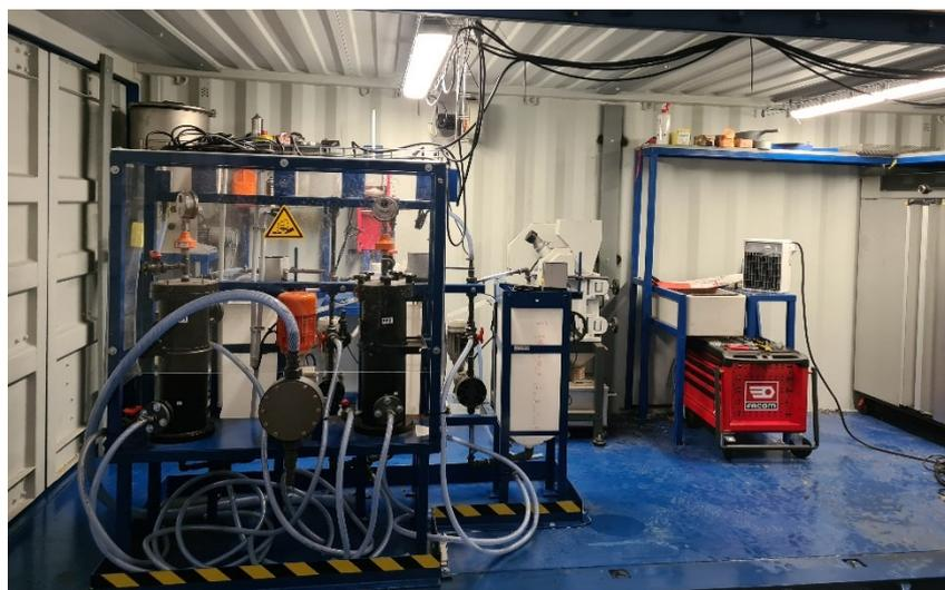
Figure 3.4.21: PULSE demonstrator: drying, crushing, leaching, precipitation, and filtration modules installed inside container (Picture: ULiège/ Z. Shariff).
