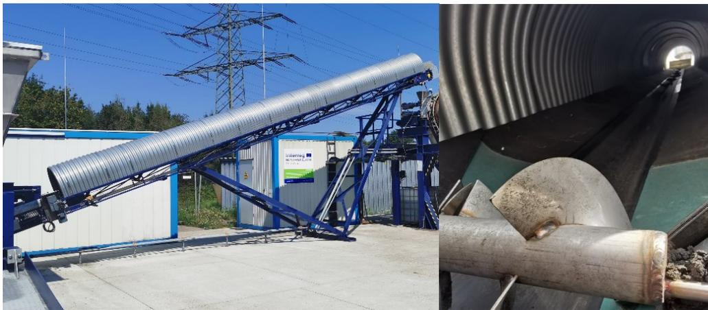
Figure 3.2.5 a and b: Conveyor belt and rotating cutter (Pictures: Emschergenossenschaft/L. Pamuk)
