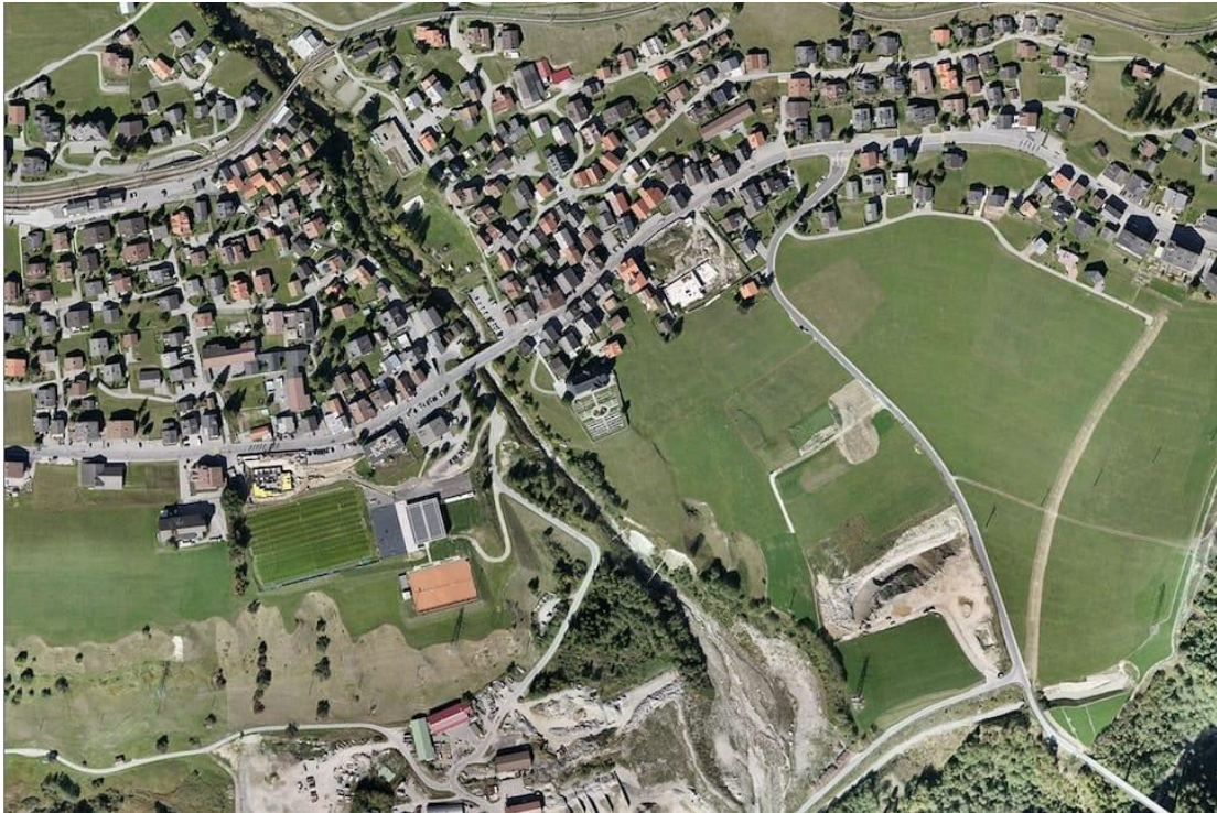
Fig.12 Orthomosaic maps. Drone images are corrected for image distortion and stitched together during post-processing to create a highly accurate orthomosaic map. Each pixel contains 2D geo-information (X, Y) and can directly procure accurate measurements, such as horizontal distances and surfaces. (Image:
