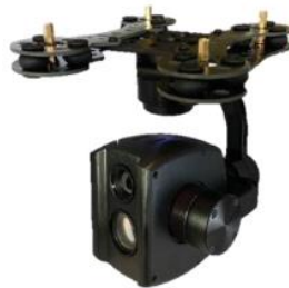
Fig.31 Thermal camera SMT18HT6 combines 18x optical zoom and 640 x 480 thermal imaging system
