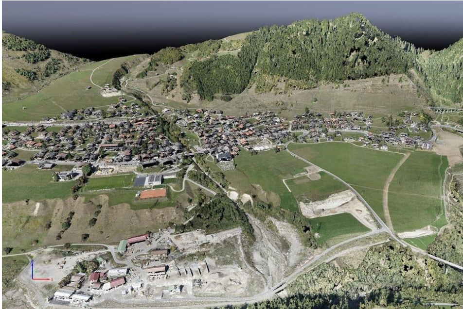
Fig.13 A densified point cloud can be generated from drone images. Each point contains geospatial (X, Y, Z) and color information. It provides a very accurate model for distance (slant and horizontal), area and volume measurements. (Image: by Wintgra, https://wingtra.com )
