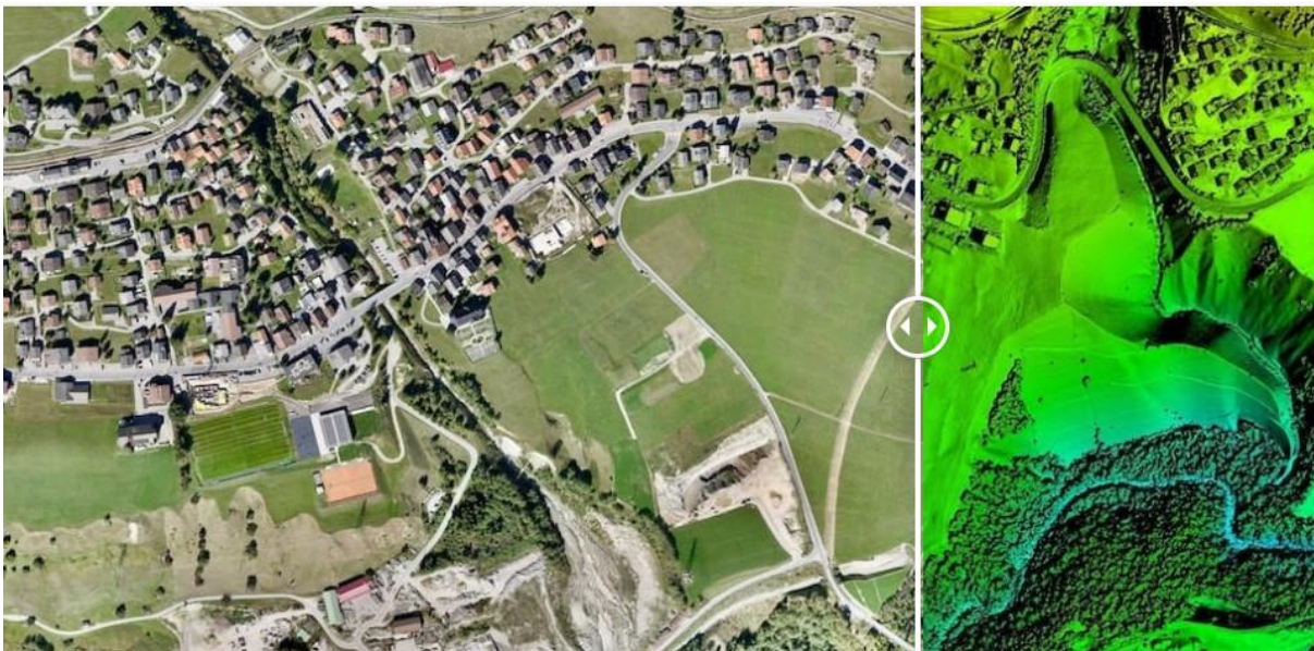
Fig.3 Orthomosaic and digital surface model created from aerial images taken by the WingtraOne surveying and mapping drone. (Image: By Wintgra, https://wingtra.com )
