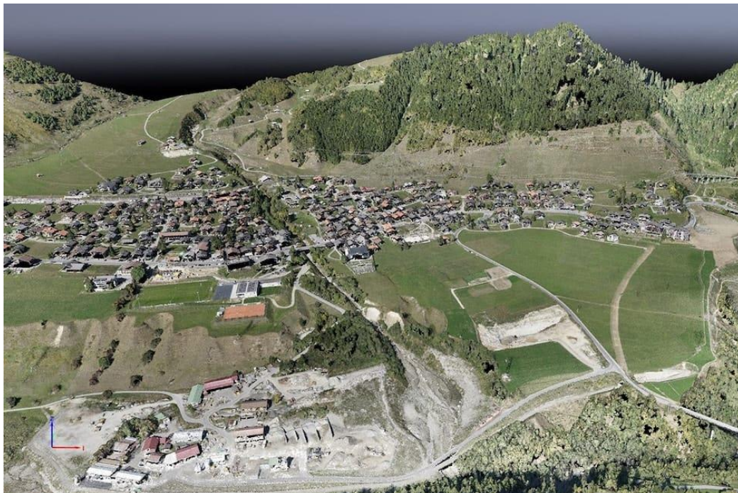
Fig.16 The 3D textured mesh is a reproduction of the edges, faces, vertices and texture of the area shot by the drone. This model is most useful for visual inspection or for when external stakeholders or public involvement is essential for a project. (Image: by Wintgra, https://wingtra.com )
