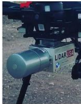
Fig.20 The Snoopy LidarUSA LIDAR camera, shot at 700,000 dots / s, has 32 individual lasers with a range of -40 degrees vertical and 360 degrees horizontal flax, +/- 2 cm accuracy and 100 m range
