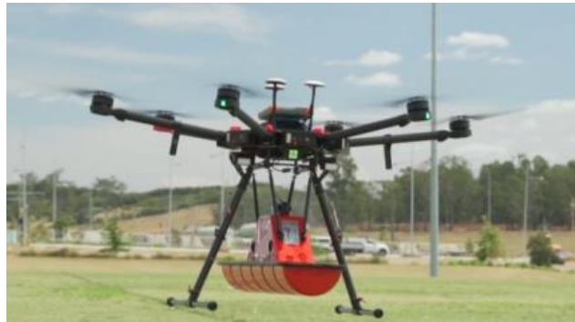
Fig.37 COBRA DJI Matrice600 Pro with georadar (GPR) uses real-time radar signal
