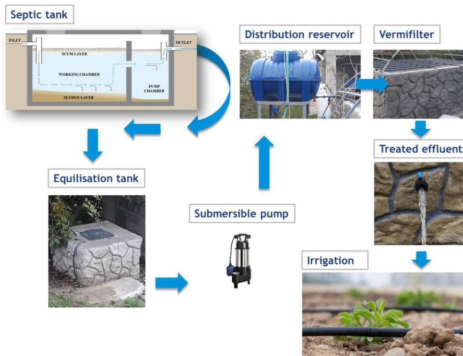
Figure 15. A schematic view of a demonstration vermifiltre built by WiSDOM association in a rural area of Moldova, at household level
