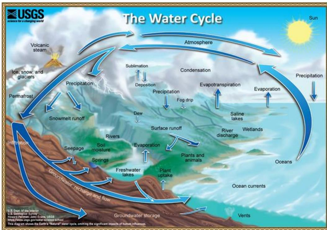
Figure 1. The natural water cycle<sup>1</sup>
