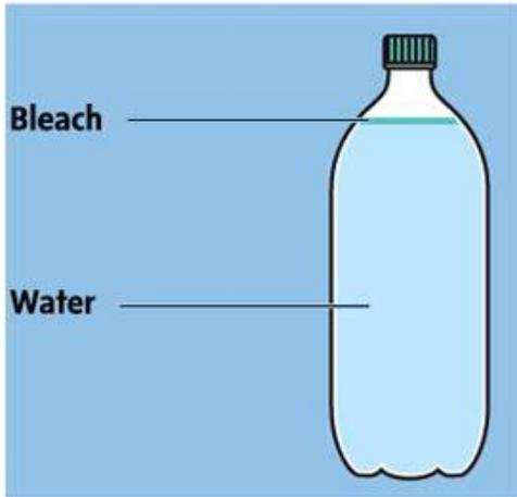
The water light bulb is simple and cheap. A 2-litre bottle is filled with clean water, plus about 10 millilitres of bleach in order to inhibit algae growth over time.
