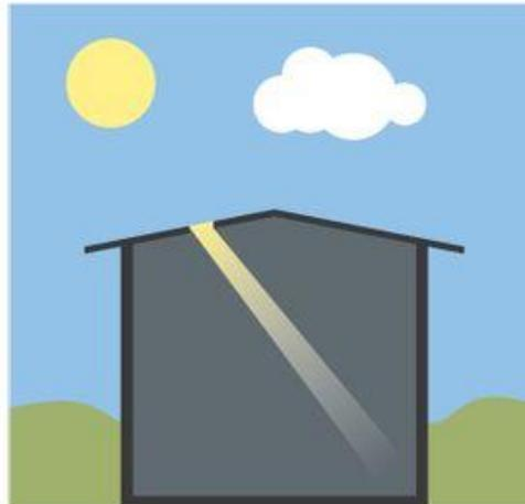
The advantage to using solar water bulbs over simply cutting holes in the roof is that sunlight shining down a hole works like a spotlight, lighting only a small area within the room.
