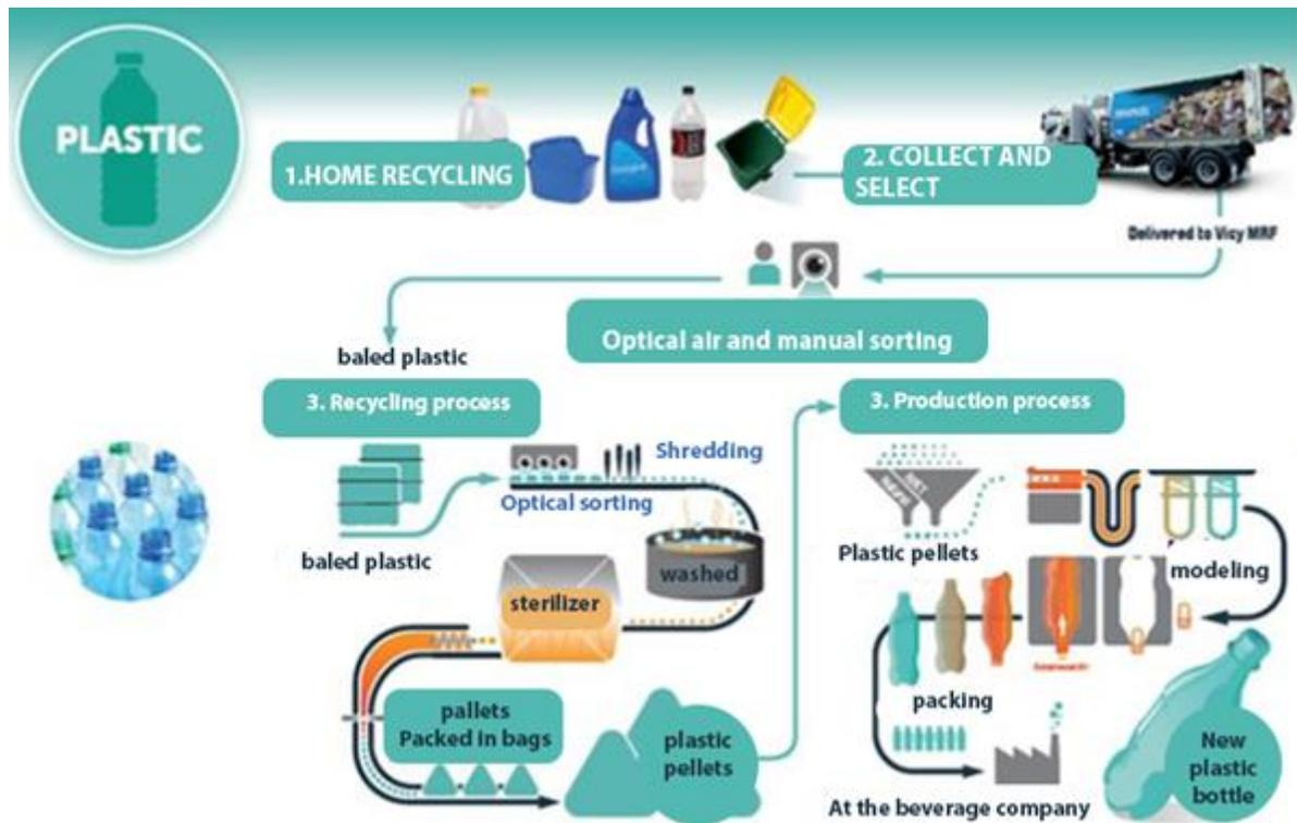
Figure 18. The cycle of recycling and recovery of plastic.
