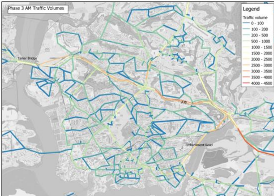
Fig. 28: Traffic flow volumes on model links (Phase 3, UK Max scenario, AM peak period)
