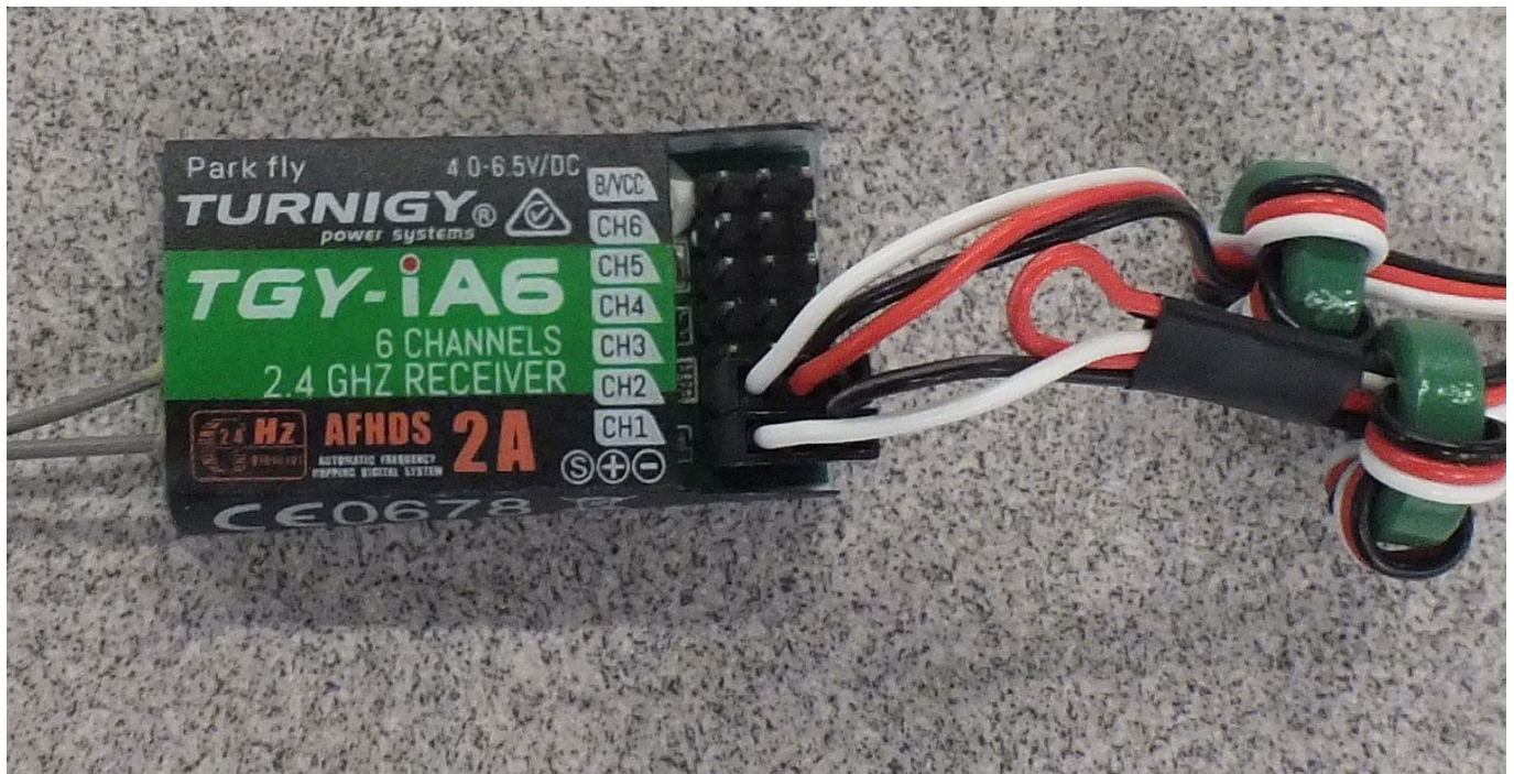
Receiver Unit showing motor connections
