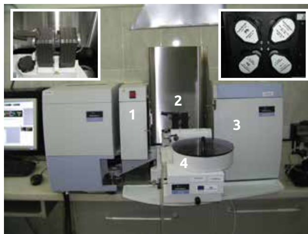
Fig. 2.10. AAAnalyst 400 atomic absorption spectrometer: 1 – spectrometer; 2 – electrothermal atomization furnace with graphite reservoir; 3 – carousel with 4 lamps; 4 – autosampler AS-800.
