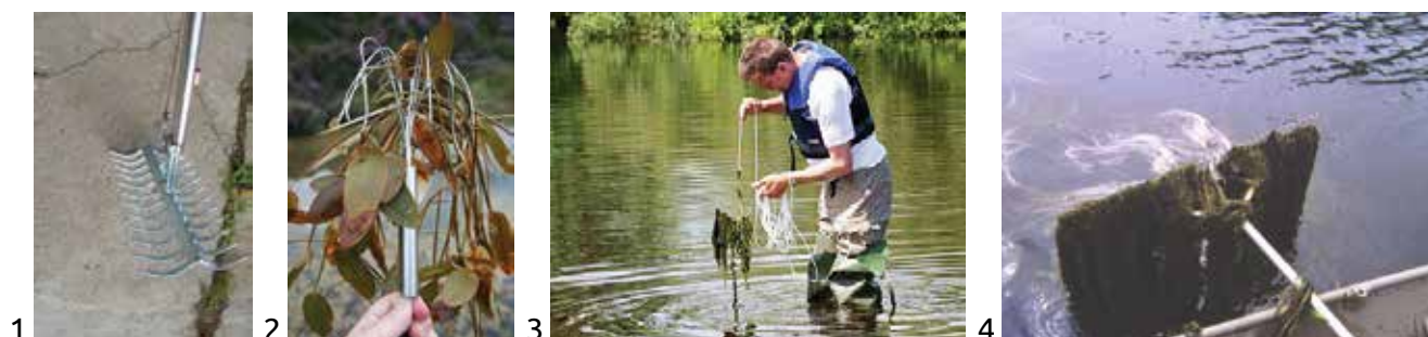
Fig. 6.4: 1 – a type of rake-grapnel 12 ; 2 – grapnel with few arms 13 ; 3 – sampling of macrophytes with a grapnel 14 ; 4 – usage of a rake-grapnel 15
