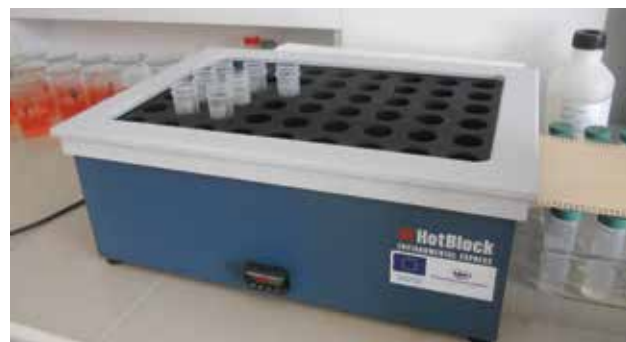
Fig. 2.9. Digester with graphite mattress HotBlock SC 151
