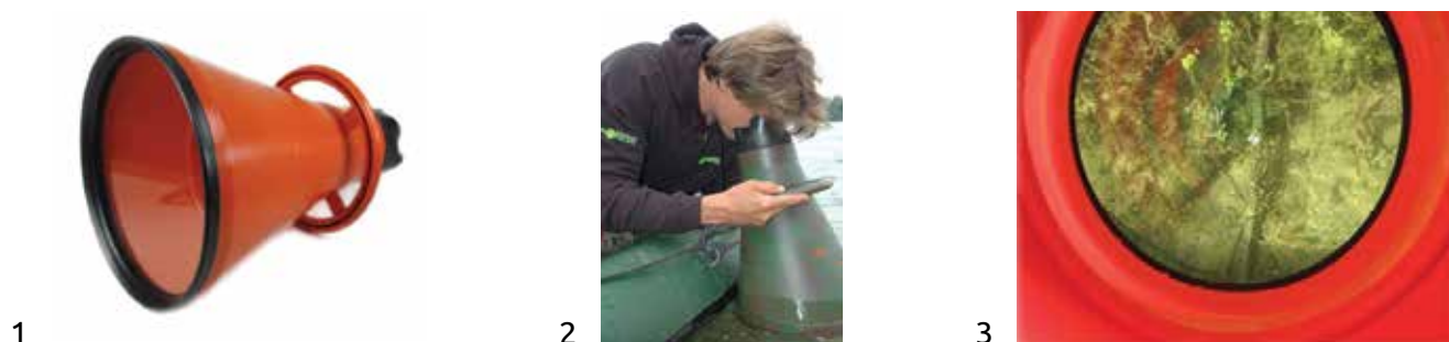
Fig. 6.2. Hydroscope: 1 – aspect 7 , 2 – mode of usage 8 , 3 – obtained image 9
