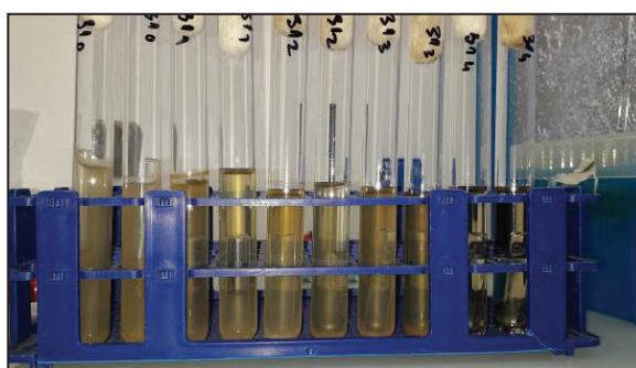
Figure 3.15. The method of multiple tubes: Positive tubes of the confirmatory test after incubation at 37 °C for 48 hours
