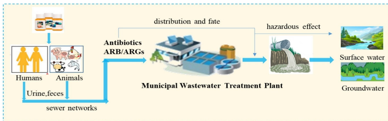
Figure 3.2. The route of ARB and ARGs in correlation with antibiotics dispersion in aquatic environments (after Wang et al., 2020)
