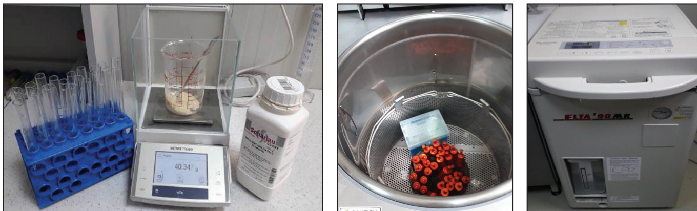
Figure 3.9. Preparing culture media, a - weighing and dosing of culture media, b - sterilization of culture media and pipette tips
