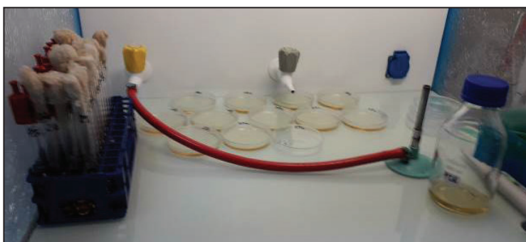
Figure 3.11. Omogenization of the dilution samples with culture media in sterile Petri dishes
