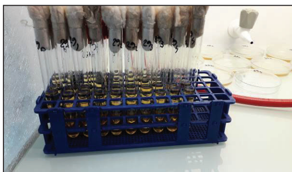
Figure 3.12. The method of multiple tubes: Inoculation of the sample dilutions in specific medium for presumptive test
