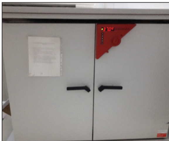
Figure 3.13. The incubation of the Petri dishes and tubes with the sample dilutions at 37 °C for 48 hours
