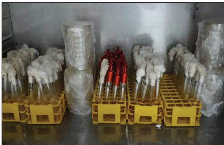
Figure 3.13. The incubation of the Petri dishes and tubes with the sample dilutions at 37 °C for 48 hours
