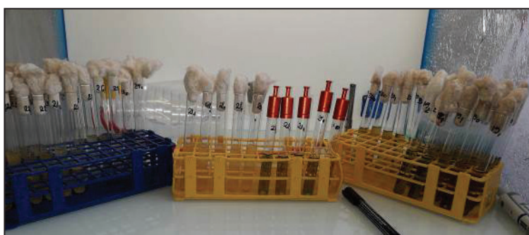
Figure 3.14. Multiple tubes method: inoculation from positive test specific medium for confirmatory test
