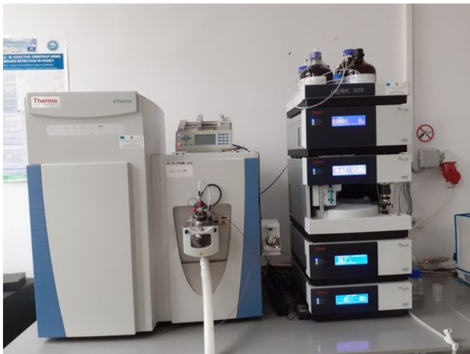
Figure 7.2. Q-Exactive Orbitrap high resolution mass spectrometer
