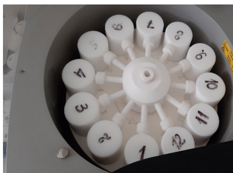
b. Microwave digester, for solid and semi-liquid samples, SpeedWave four SW-4 (Berghof).
