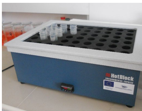
a. Liquid sample digester, HotBlock SC 151 (Environmental Express);
