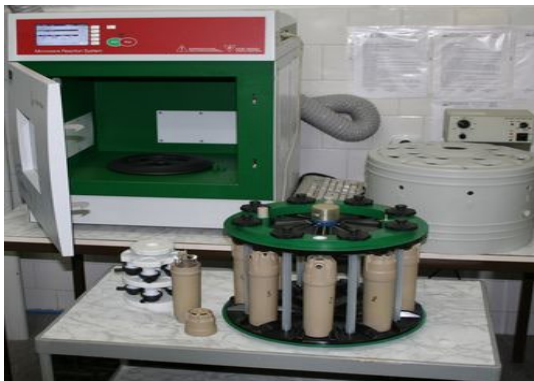
Figure 5.9. Microwave Oven Anton Paar (DDNI)
