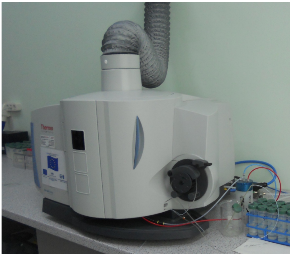
Figure 4.2. Thermo Scientific iCAP 6200 Duo atomic emission spectrometer.
