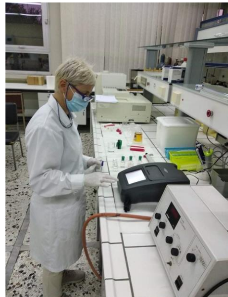
Fig. 2.10. Environmental samples analysis with UV-Vis spectrophotometer [15]
