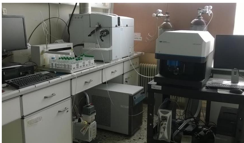
Σχήμα 1.18. LA-ICP-MS, ICP-MS Agilent 7700X coupled with LA Teledyne LSX-213 G2 [16]
