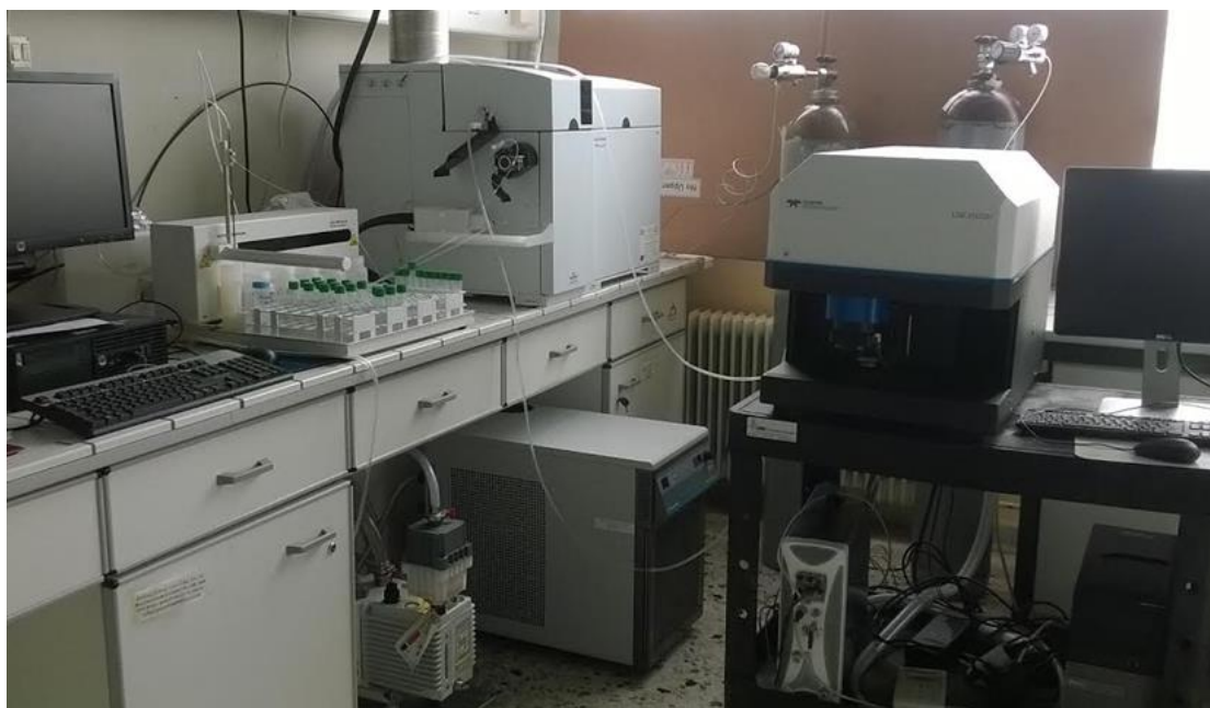
Fig. 1.18. LA-ICP-MS, ICP-MS Agilent 7700X coupled with LA LSX-213 G2 Teledyne [16]
