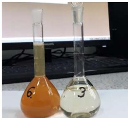
**Figure 3. Representative color change for ammonia content in treated and untreated wastewater**
